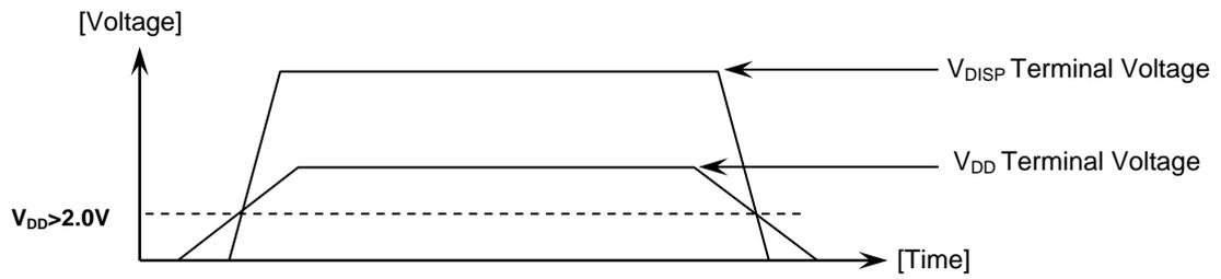
To prevent IC from malfunctioning,  $V_{DISP}$  should be applied after  $V_{DD}$  is applied.
