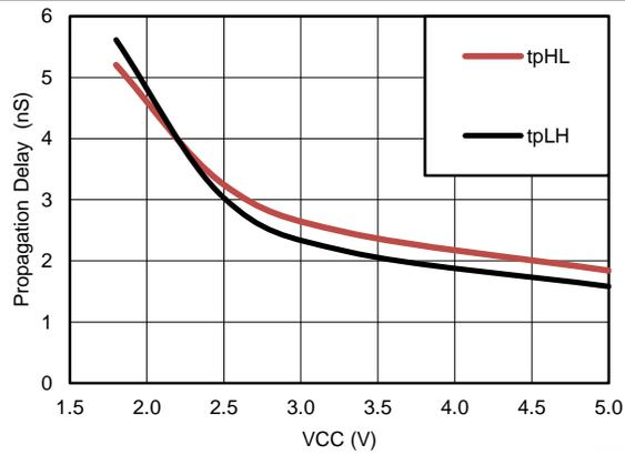
Figure 1. Propagation Delay vs. V<sub>CC</sub>
