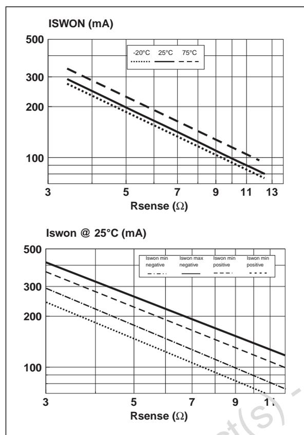
The choice of the switching-on current is function of the  $R_{SENSE}$  resistors.
