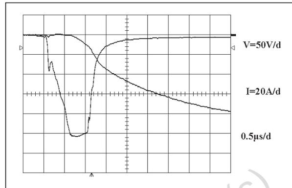
Figures 14 and 15 show that the remaining overvoltage does not exceed  $\pm 260$  V. The CLP200M switches on within  $0.7 \mu s$  and withstands the 100 A given by the CCITT K20 generator.
