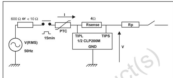
**Fig. 20 :** Power contact test 3 (With 10 $\Omega$  series).
