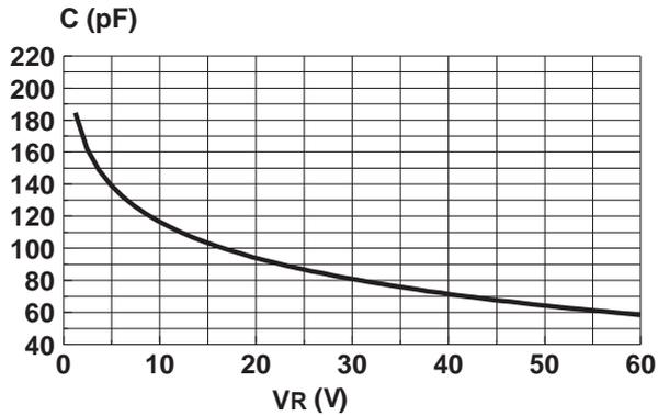
**Fig. 38 :** Typical and maximal capacitance between TIPL, RINGL and GND.
