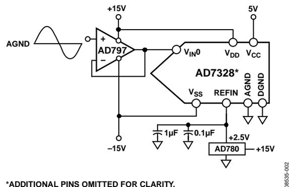
Figure 2. Single-Ended Input Operation (Simplified Schematic: Decoupling and All Connections Not Shown)
