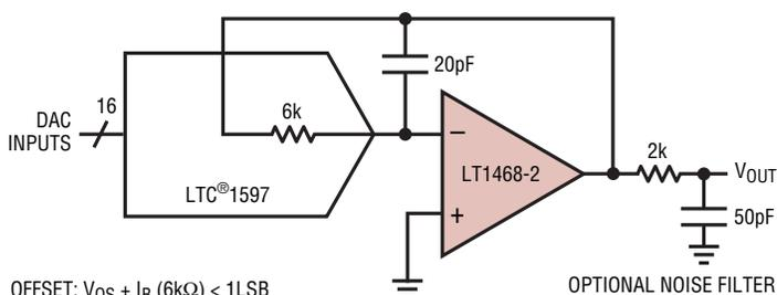
OFFSET:  $V_{OS} + I_B (6k\Omega) < 1\text{LSB}$
