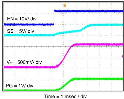
Figure 40. TPS563219A Start Up Relative To EN
