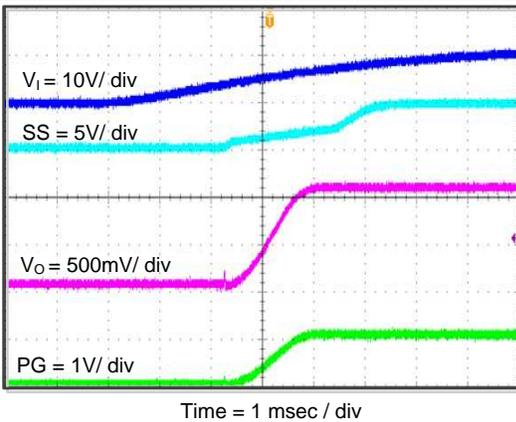
Figure 39. TPS563219A Start Up Relative To V<sub>1</sub>
