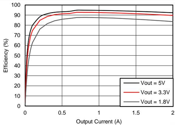
Figure 5. Efficiency vs Output Current
