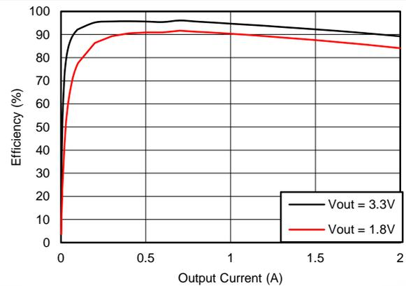
Figure 6. Efficiency vs Output Current ( $V_i = 5V$ )
