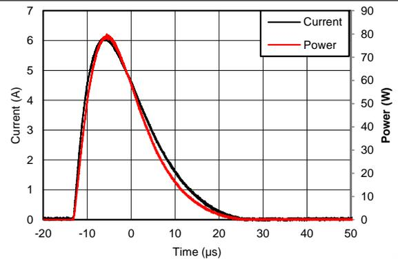
**Figure 8. Surge Curve ( $t_p = 8/20\ \mu\text{s}$ )
