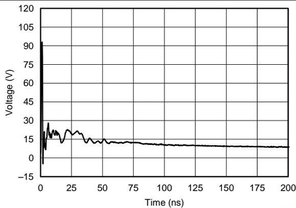
Figure 3. IEC 61000-4-2 Clamping Voltage, 8-kV Contact
