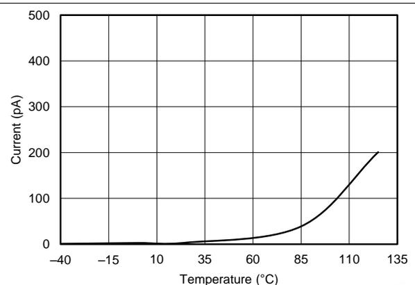
Figure 6.  $I_{\text{LEAK}}$  vs Temperature,  $V_{\text{IN}} = 2.5 \text{ V}$
