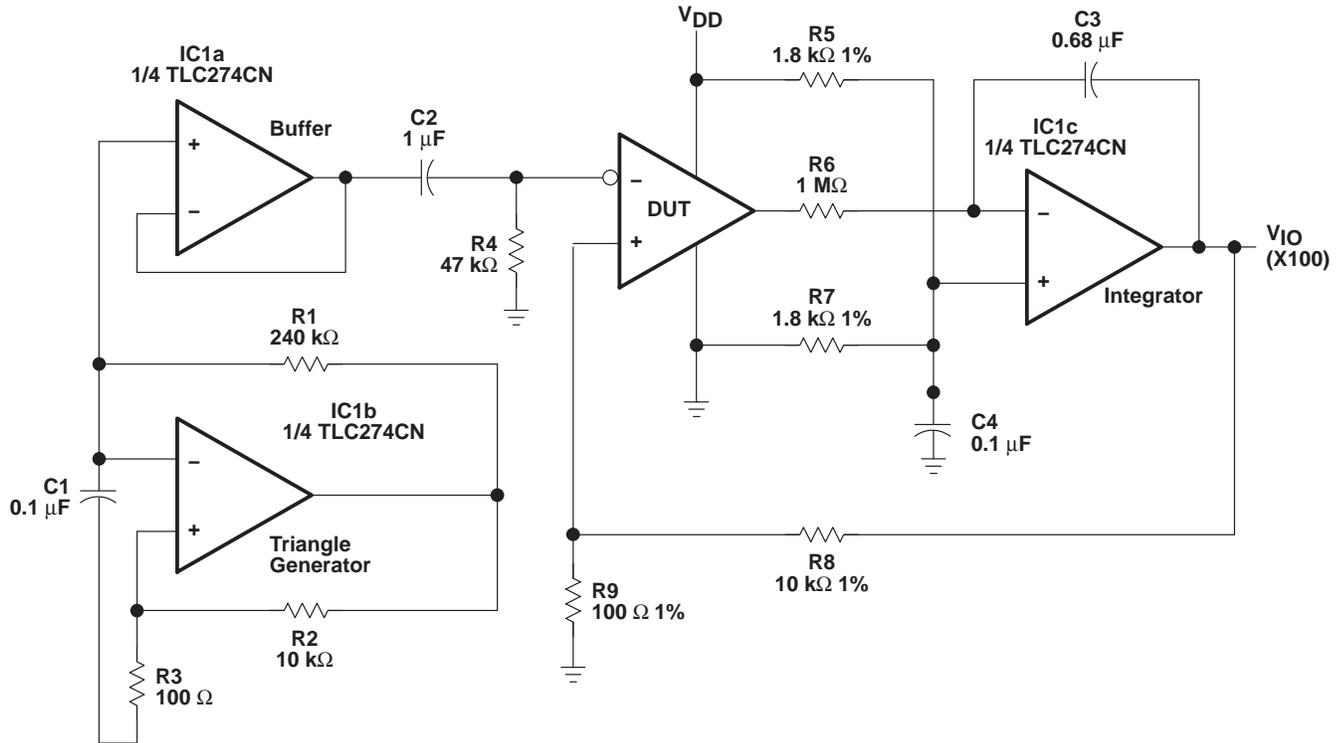
**Figure 6. Circuit for Input Offset Voltage Measurement**
