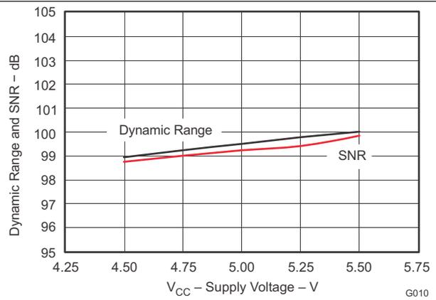
Figure 16. Dynamic Range and SNR vs Supply Voltage
