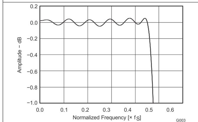
**Figure 9. Decimation-Filter Frequency Response Pass-Band Ripple Characteristics**
