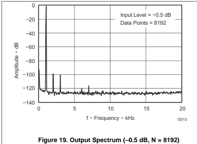
Figure 19. Output Spectrum (-0.5 dB, N = 8192)
