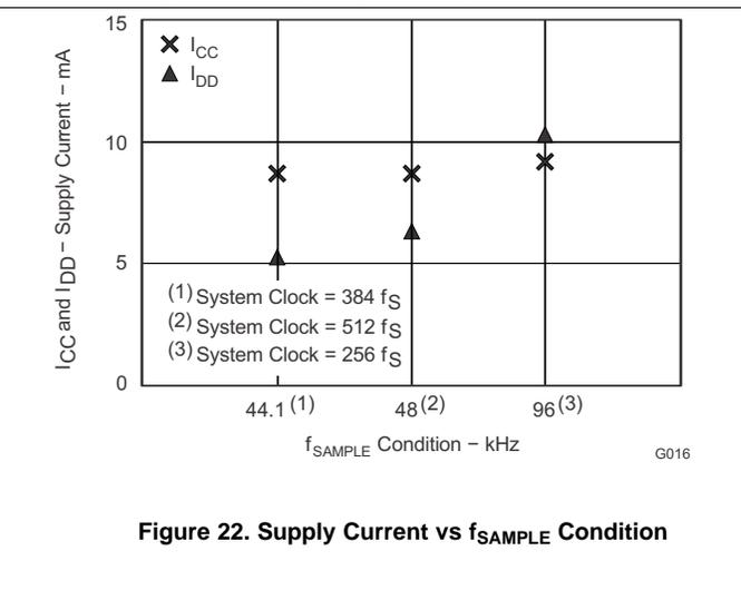
Figure 22. Supply Current vs  $f_{\text{SAMPLE}}$  Condition
