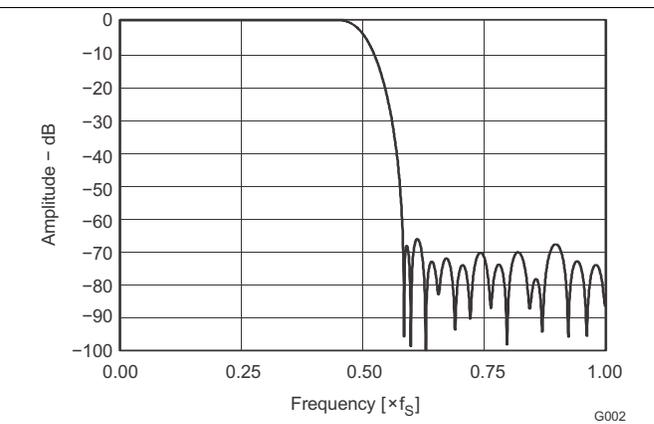
**Figure 8. Decimation-Filter Frequency Response Stop-Band Attenuation Characteristics**
