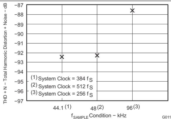
Figure 17. THD+N vs  $f_{SAMPLE}$  Condition
