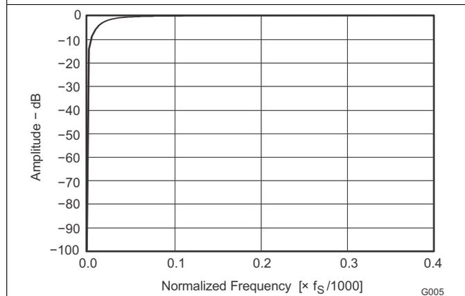
**Figure 11. High-Pass Filter Frequency Response HPF Stop-Band Characteristics**
