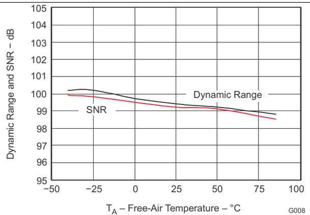
Figure 14. Dynamic Range and SNR vs Temperature
