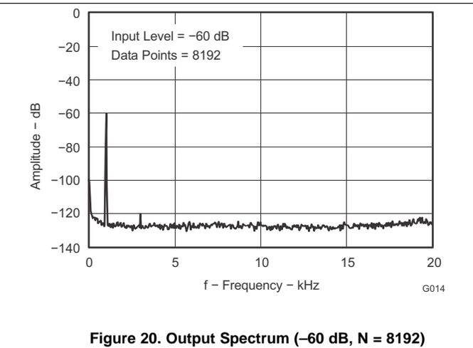
Figure 20. Output Spectrum (-60 dB, N = 8192)
