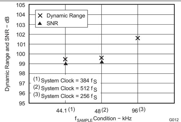
Figure 18. Dynamic Range and SNR vs  $f_{SAMPLE}$  Condition
