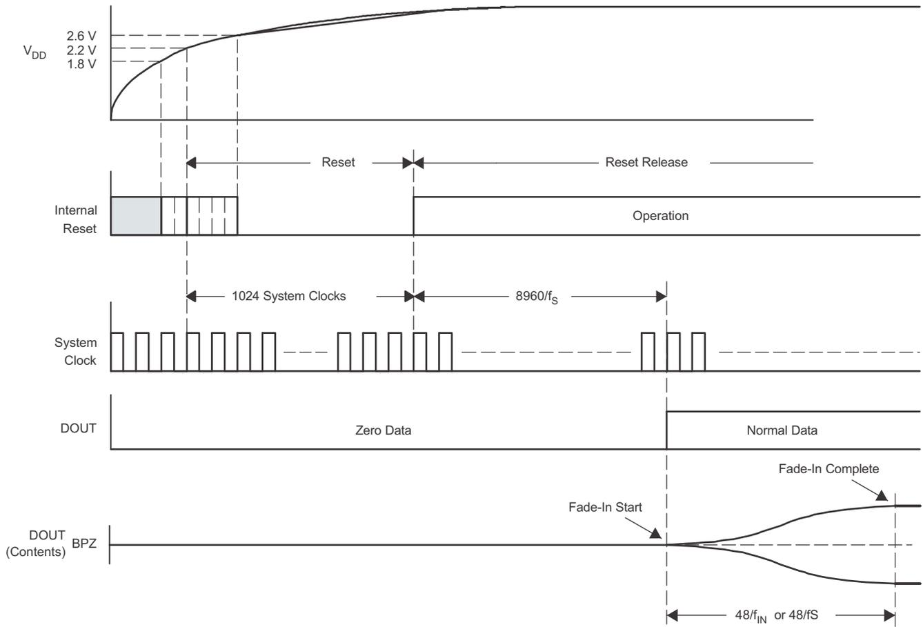
**Figure 2. Power-On Timing**
