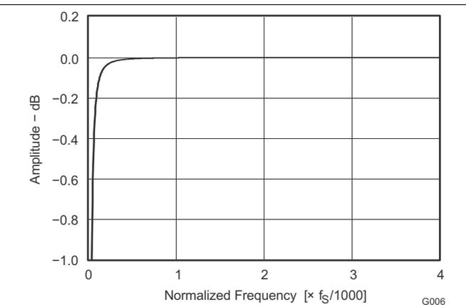
**Figure 12. High-Pass Filter Frequency Response HPF Stop-Band Characteristics**
