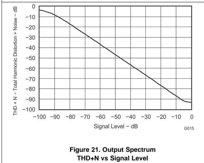
Figure 21. Output Spectrum THD+N vs Signal Level
