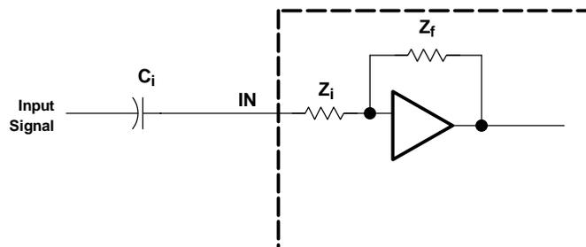
The -3-dB frequency can be calculated using Equation 4.
