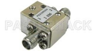
Isolator with 18 dB Isolation from 7 GHz to 12.4 GHz, 10 Watts and SMA Female
