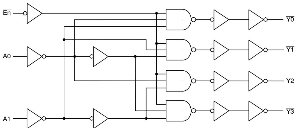
Figure 4. Expanded Logic Diagram
