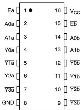
Figure 1. Pin Assignment
