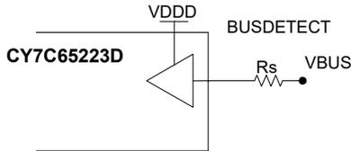
When VBUS > VDDD, a resistor voltage divider is necessary to reduce the voltage from VBUS down to VDDD for the GPIO sensing the VBUS voltage. This is shown in Figure 9. The resistors should be sized as follows:
