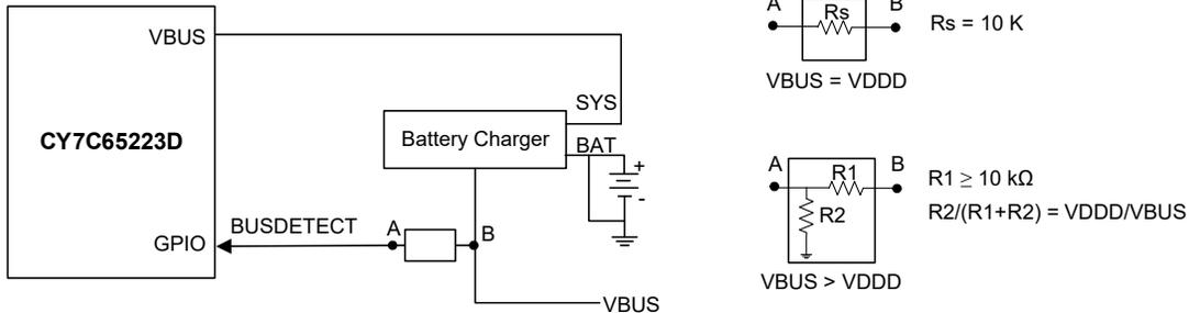
When VBUS and VDDD are at the same voltage potential, VBUS can be connected to GPIO using a series resistor ( $R_s$ ). This is shown in Figure 8. If there is a charger failure and VBUS becomes 9 V, then the 10-k $\Omega$  resistor plays two roles. It reduces the amount of current flowing into the forward biased diodes in the GPIO, and it reduces the voltage seen on the pad.
