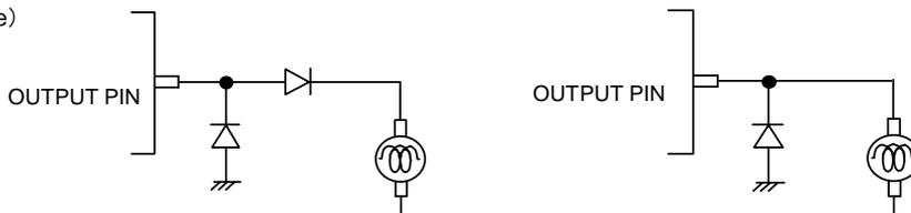
8. In the application , in case of the each terminal is lower than Gnd , it recommend to use the bypass circuit.
