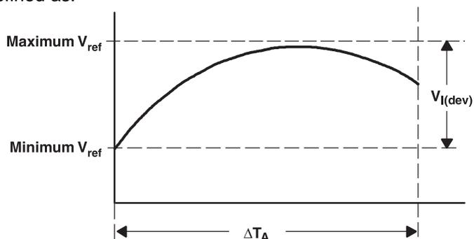
$\alpha_{V_{ref}}$  is positive or negative, depending on whether minimum  $V_{ref}$  or maximum  $V_{ref}$ , respectively, occurs at the lower temperature. The full-range temperature coefficient is an average and therefore any subsection of the rated operating temperature range can yield a value that is greater or less than the average. For more details on temperature coefficient, check out [Voltage Reference Selection Basics](#).
