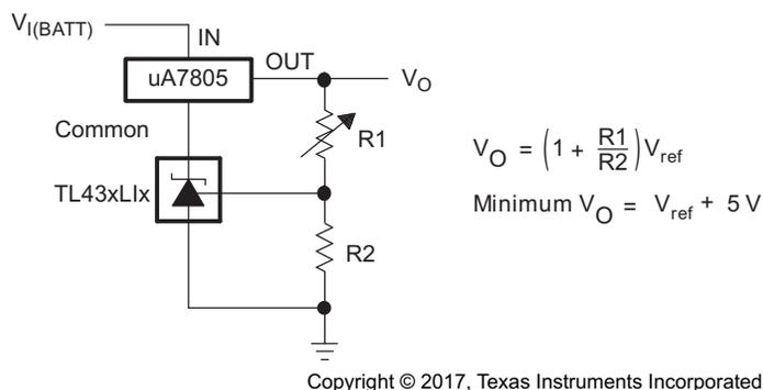
**Figure 28. Output Control of a Three-Terminal Fixed Regulator**
