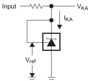
Figure 14. Test Circuit for  $V_{KA} = V_{ref}$
