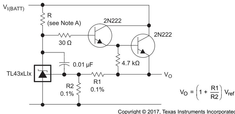
A. R should provide cathode current  $\geq 1$  mA to the TL431LI at minimum  $V_{(BATT)}$ .
