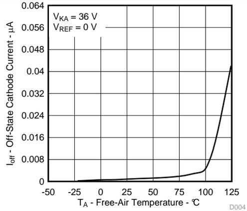
Figure 4. Off-State Cathode Current vs Free-Air Temperature
