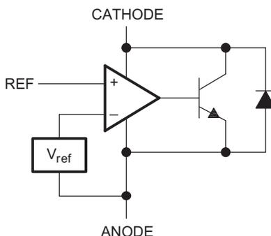
Figure 18. Equivalent Schematic
