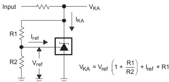
Figure 15. Test Circuit for  $V_{KA} > V_{ref}$
