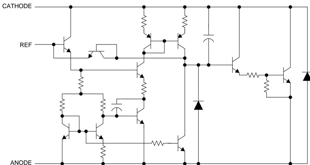
Figure 19. Detailed Schematic
