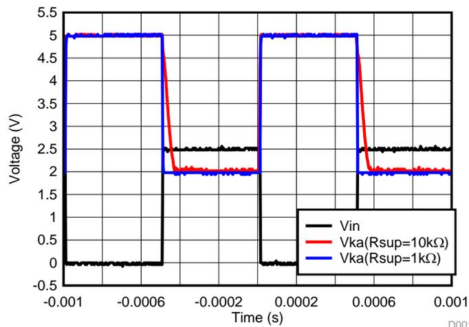
Figure 21. Output Response With Various Cathode Currents
