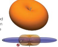
Gain is also related to the overall physical size of the antenna, as well as surrounding materials. As the geometry of the antenna is reduced below the effective wavelength (considered an electrically small antenna) the gain decreases. Also, the relative distance between an electrically small antenna and its associated ground impacts antenna gain.
