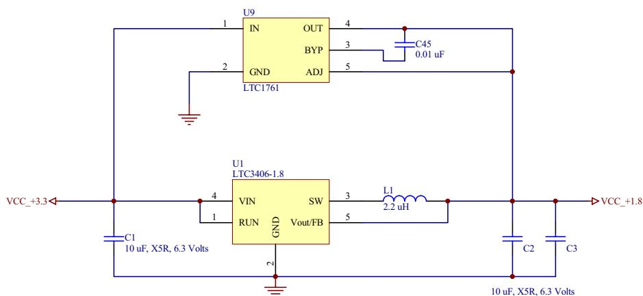
This is a simple switching regulator. It produces 1.8V at >500 mA at about 90% efficiency. A simple low drop out linear regulator would be a cheaper alternative at the expense of power. A linear regulator would dissipate about 0.75 watts max. This switching regulator dissipates about 0.10 watts max.
