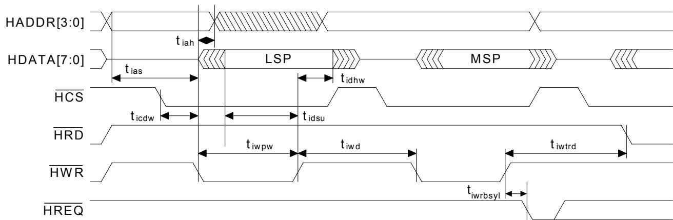
**Figure 17. Parallel Control Port - Intel Mode Write Cycle**
