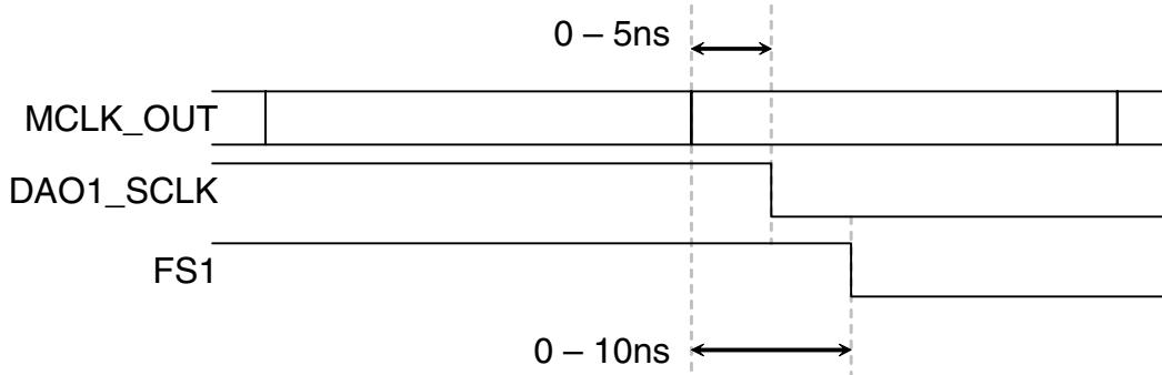
**Figure 6. Timing Relationship between FS512\_OUT, DAO1\_SCLK and FS1**
