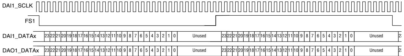
**Figure 11. Audio Data Timing Detail - I<sup>2</sup>S Mode, 128FS - CS18102x & CS49612x**
