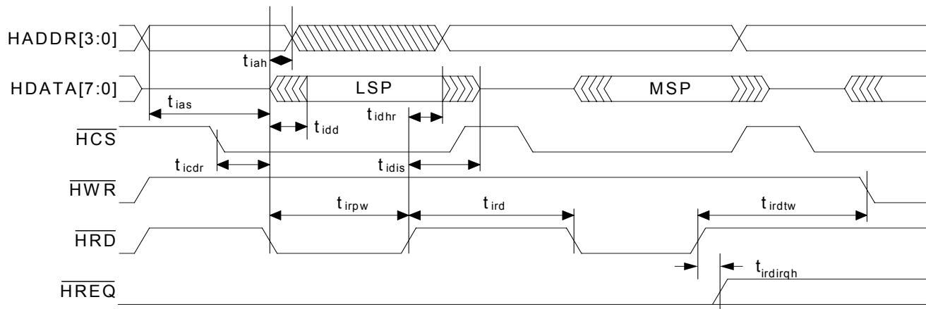
**Figure 16. Parallal Control Port - Intel Mode Read Cycle**
