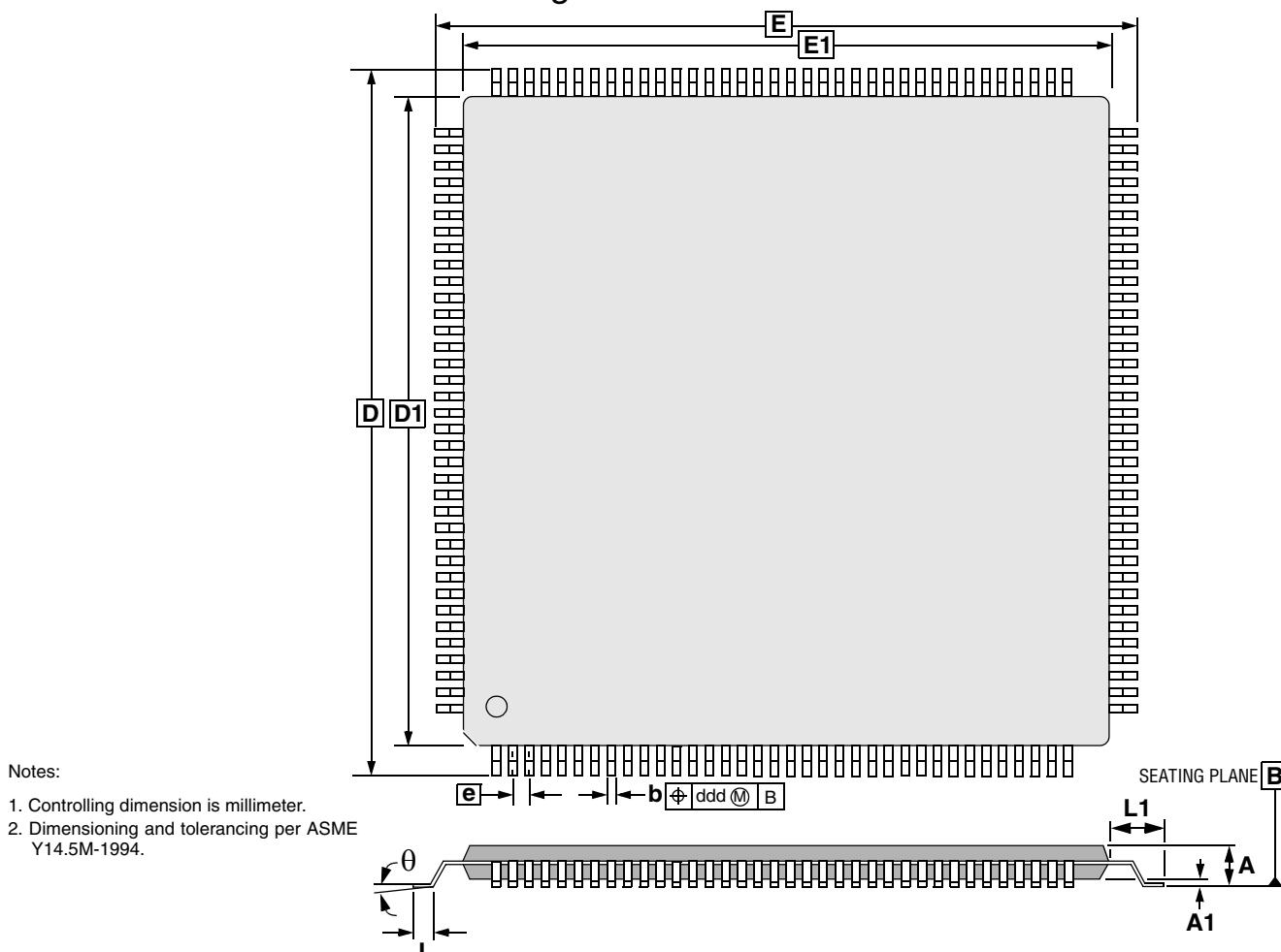
Figure 31. 144-Pin LQFP Package Drawing
