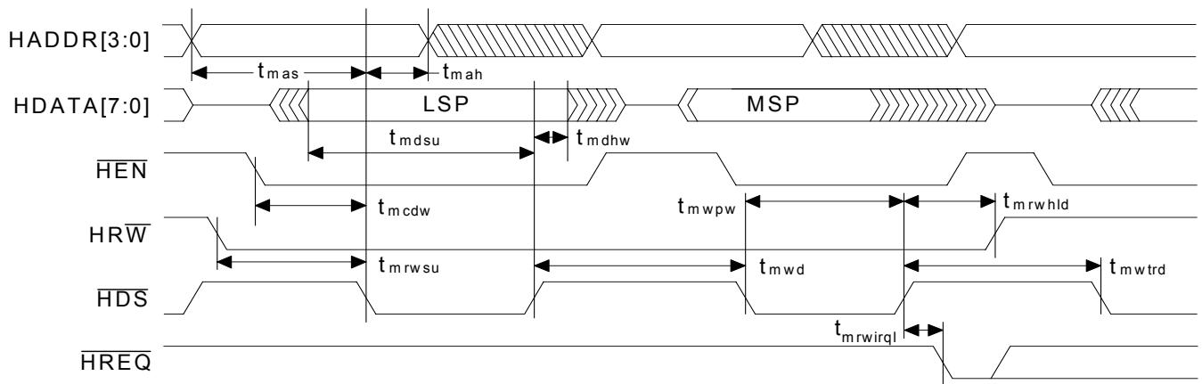
**Figure 15. Host Port Write Cycle Timing - Motorola Mode**
