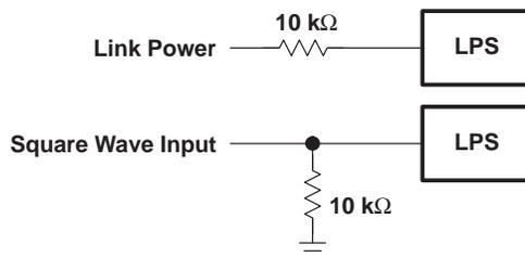
**Figure 8. Nonisolated Circuit Connection Variations for LPS**
