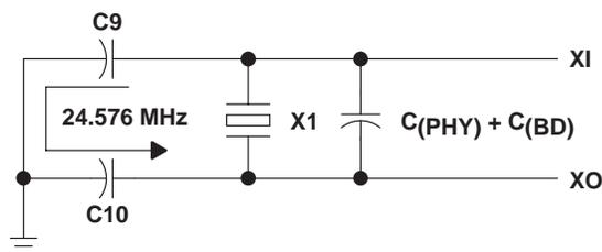
Figure 10. Load Capacitance for the TSB41AB2 PHY
