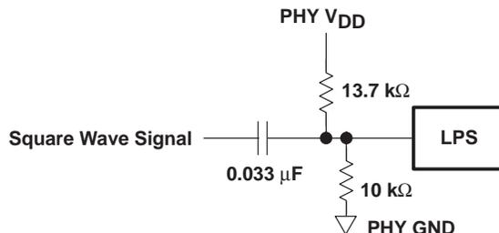
NOTE: As long as the resistance ratio is maintained between 1.61:1 and 1.33:1, any values of resistors may be used.
