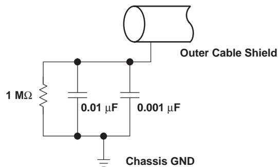
Figure 6. Compliant DC Isolated Outer Shield Termination
