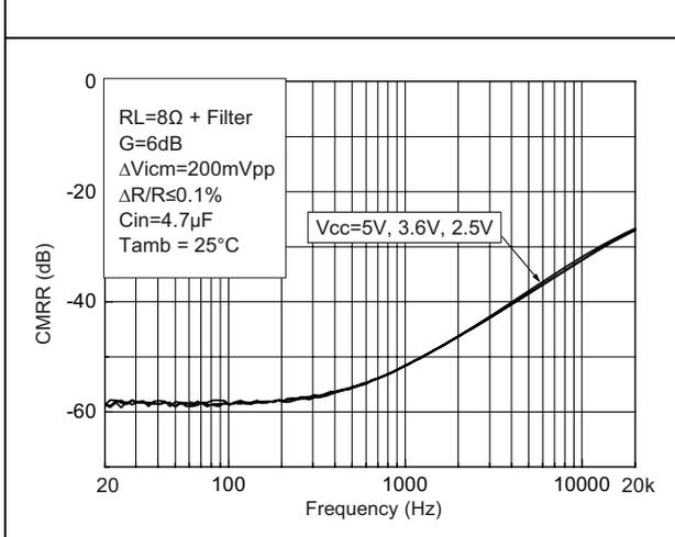
Figure 27. CMRR vs. common mode input voltage
