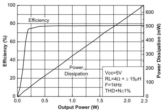
**Figure 9. Efficiency vs. output power**
