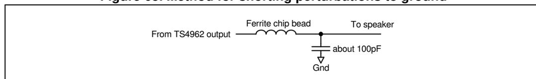
In the case where the distance between the TS4962 output and the speaker terminals is high, it is possible to observe low frequency EMI issues due to the fact that the typical operating frequency is 250 kHz. In this configuration, we recommend using an output filter (as represented in [Figure 1 on page 6](#)). It should be placed as close as possible to the device.
