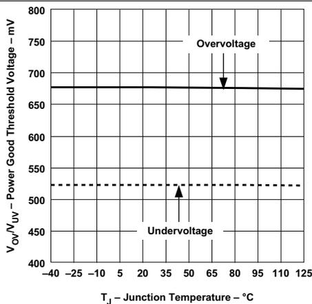
Figure 11. Power Good Threshold Voltage vs Junction Temperature
