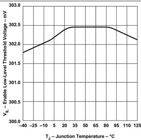
Figure 9. Enable Low-Level Threshold Voltage vs Junction Temperature
