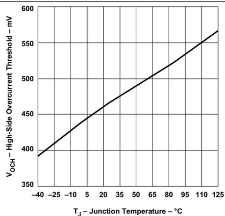
Figure 10. High-Side Overcurrent Threshold vs Junction Temperature
