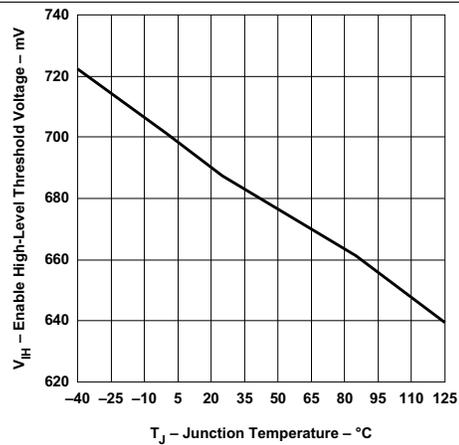
Figure 8. Enable High-Level Threshold Voltage vs Junction Temperature
