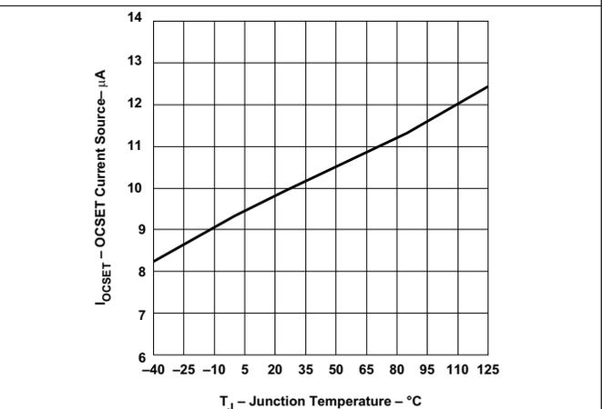
Figure 6. OCSET Current Source vs Junction Temperature
