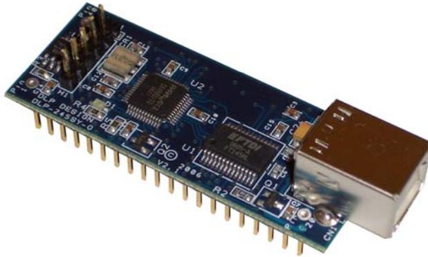
The DLP-245SY-G combines the 4<sup>th</sup> generation FT245RL USB interface IC from FTDI with a Parallax SX48 microcontroller to form a rapid development tool. The SX48 microcontroller is preprogrammed with basic functionality for accessing the port pins and can be reprogrammed with user developed firmware via a 5-pin header (4 pins used for compatibility with device programmers and debuggers from other manufacturers).
