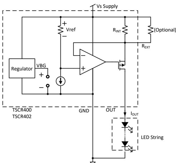
**Figure 13: Application circuit for Stand-alone current source**
