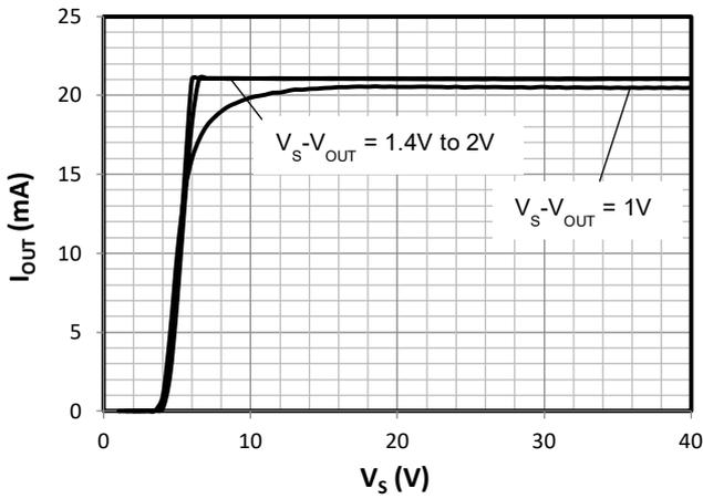
**Figure 7.  $I_{OUT}$  vs.  $V_S$**
