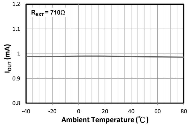
**Figure 2.  $I_{OUT}$  vs.  $T_A$  ( $R_{EXT}=710\Omega$ )**
