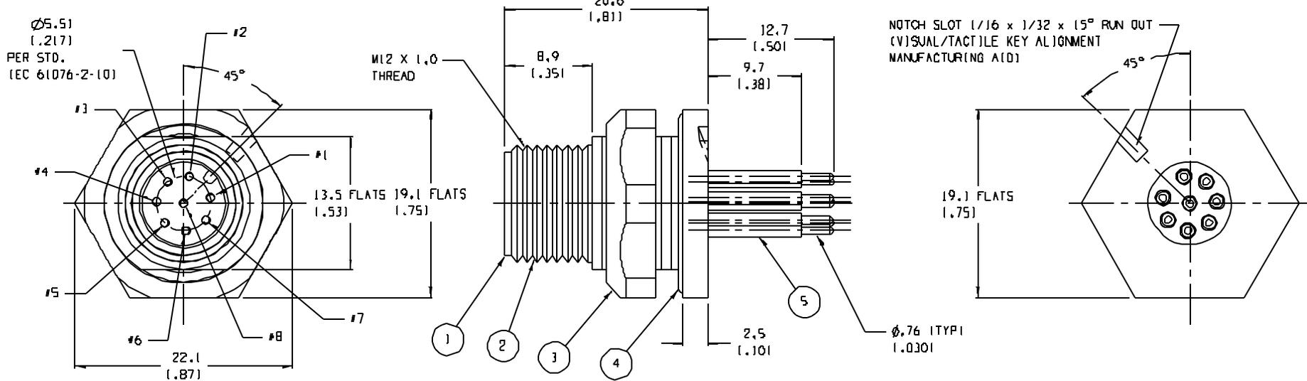
NOTCH SLOT 1/16 x 1/32 x 15° RUN OUT (VISUAL/TACTILE KEY ALIGNMENT MANUFACTURING AID)
