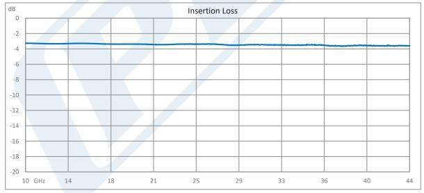
Click the following link (or enter part number in "SEARCH" on website) to obtain additional part information including price, inventory and certifications: 2 Way 2.92mm Power Divider from 10 GHz to 43.3 GHz Rated at 20 Watts PE20DV1062
