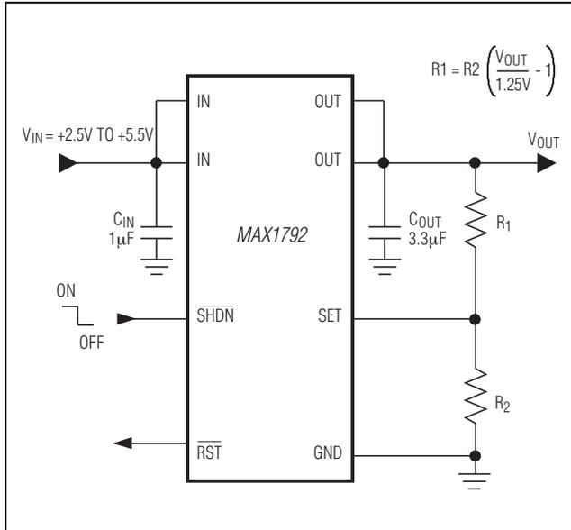
Figure 2. Adjustable Output Using External Feedback Resistors
