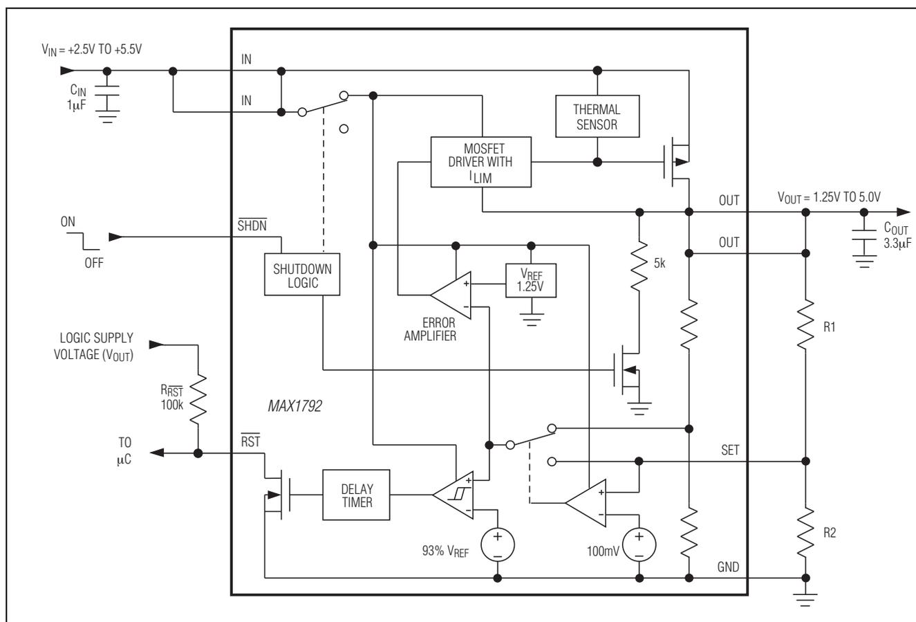
Figure 1. Functional Diagram
