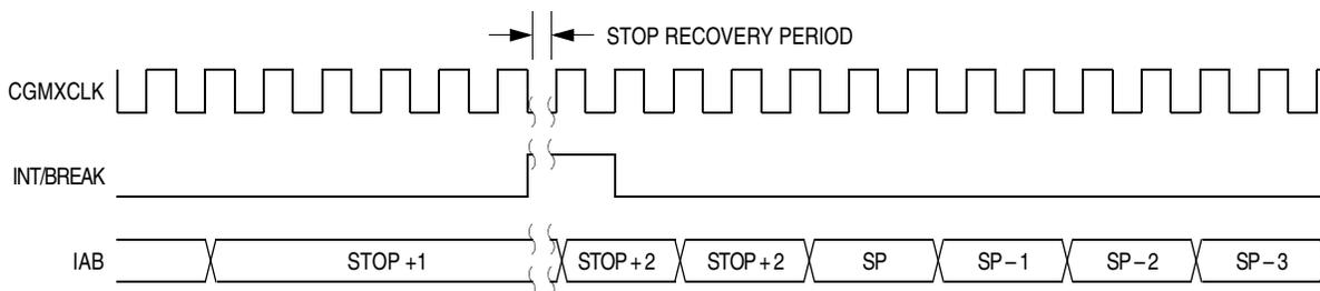
**Figure 15-16. Stop Mode Recovery from Interrupt or Break**
