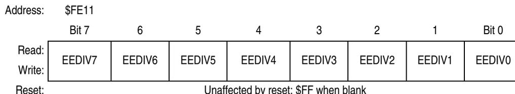
**Figure 2-10. EEPROM Divider Nonvolatile Register Low (EEDIVLNVR)**
