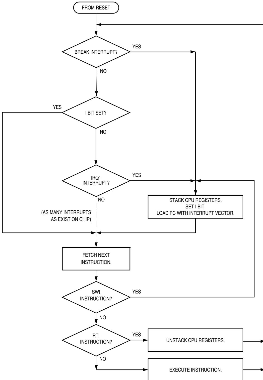
Figure 15-9. Interrupt Processing
