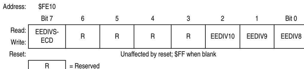
**Figure 2-9. EEPROM Divider Nonvolatile Register High (EEDIVHNVR)**
