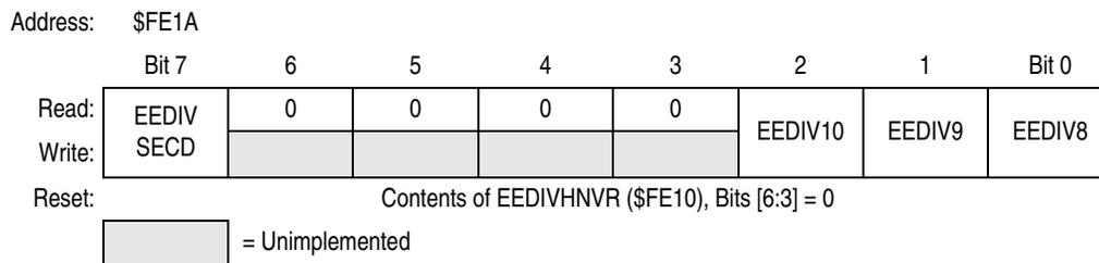
**Figure 2-7. EEDIV Divider High Register (EEDIVH)**
