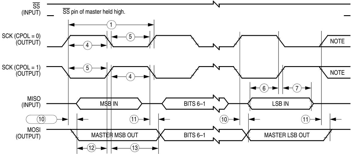
NOTE: This last clock edge is generated internally, but is not seen at the SCK pin.
