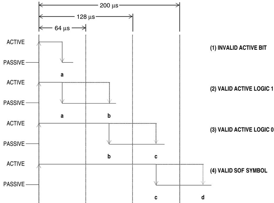
**Figure 4-10. J1850 VPW Received Active Symbol Times**
