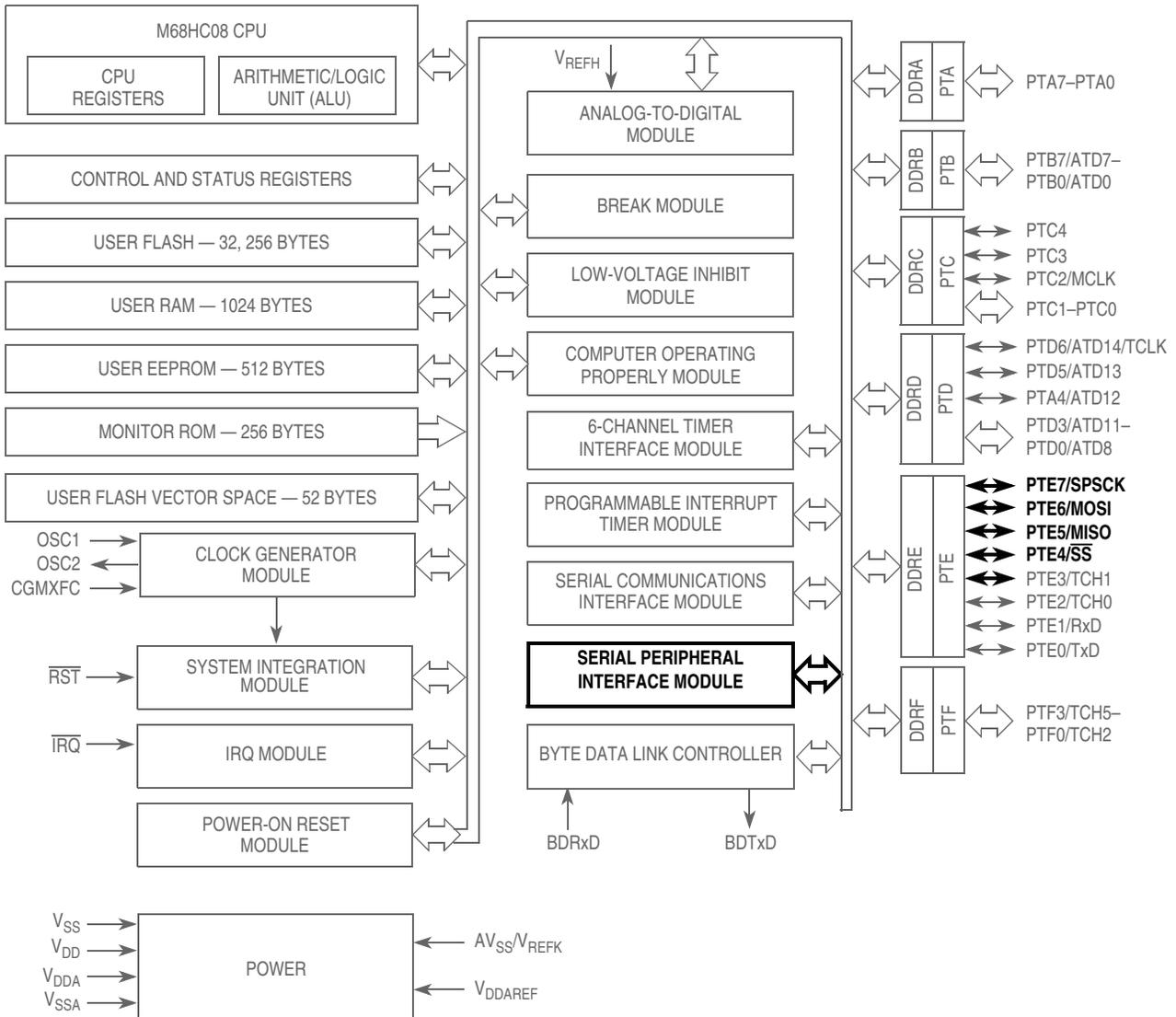
**Figure 16-1. Block Diagram Highlighting SPI Block and Pins**
