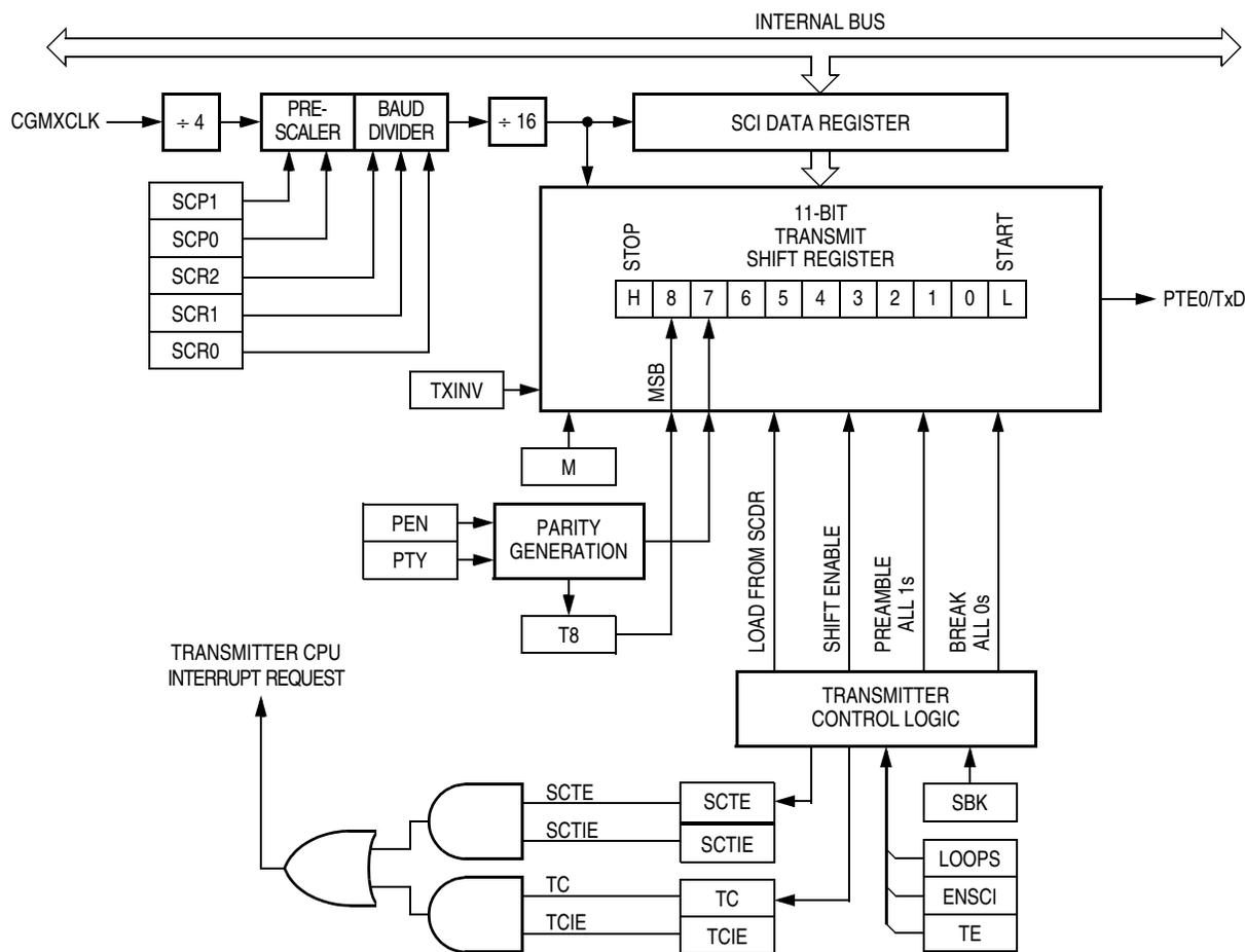
Figure 14-4. SCI Transmitter
