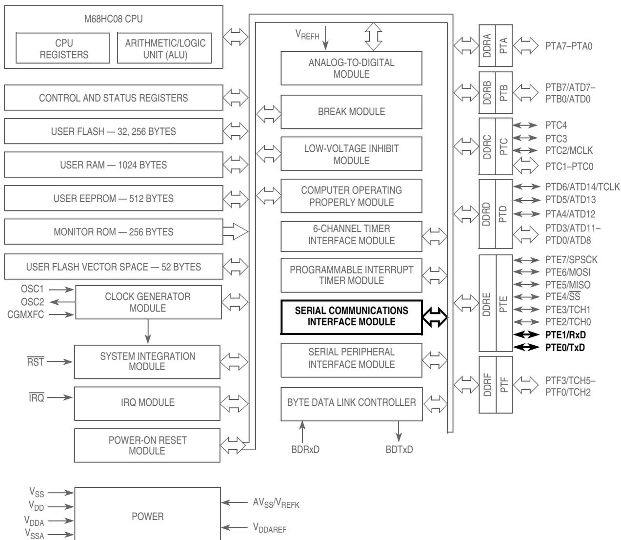
**Figure 14-1. Block Diagram Highlighting SCI Block and Pins**
