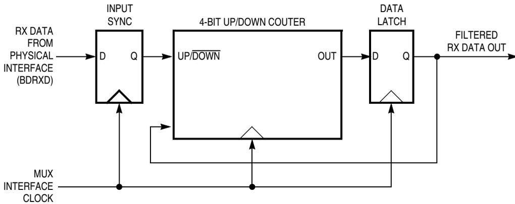
**Figure 4-5. BDLC Rx Digital Filter Block Diagram**
