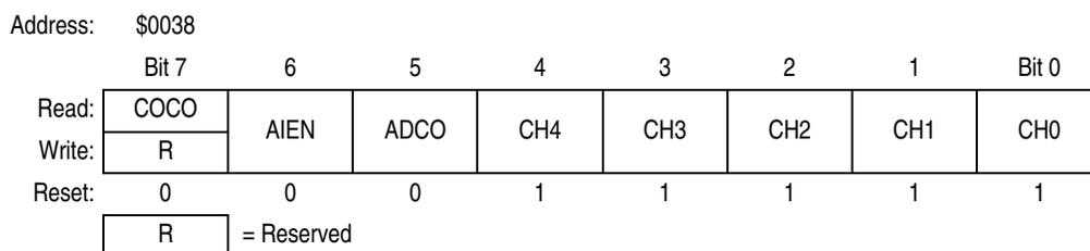
**Figure 3-3. ADC Status and Control Register (ADSCR)**
