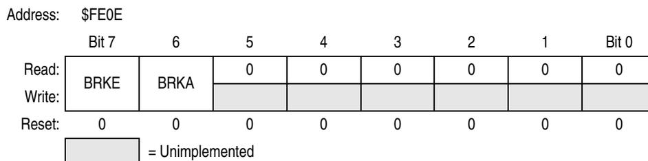
**Figure 18-3. Break Status and Control Register (BSCR)**
