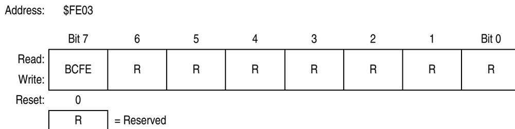
**Figure 15-19. SIM Break Flag Control Register (SBFCR)**
