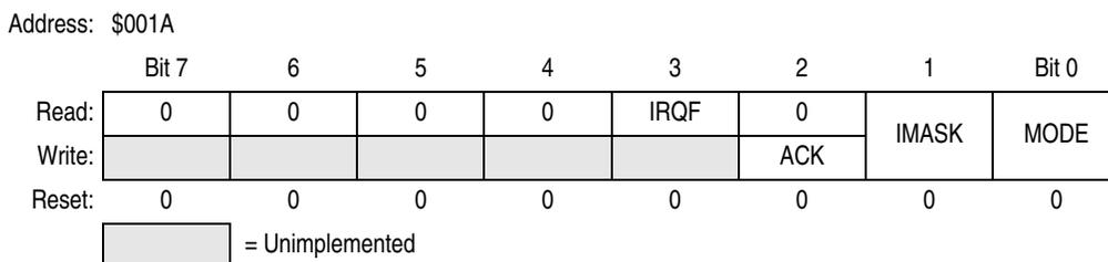
**Figure 10-4. IRQ Status and Control Register (ISCR)**
