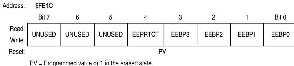
**Figure 2-6. EEPROM Nonvolatile Register (EENVR)**
