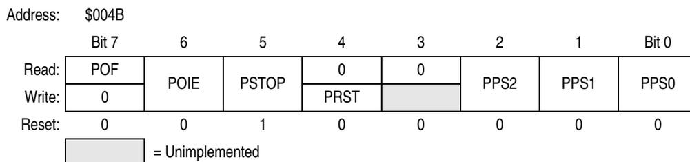
**Figure 12-2. PIT Status and Control Register (PSC)**
