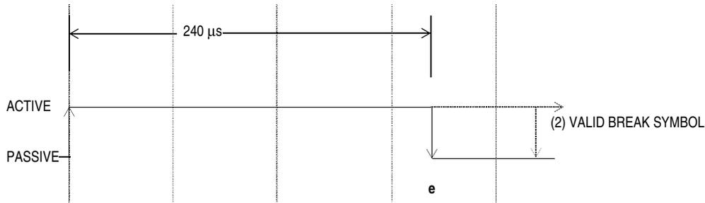
Figure 4-11. J1850 VPW Received BREAK Symbol Times
