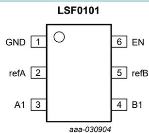
Fig. 2. Pin configuration SOT363-2 (TSSOP6)
