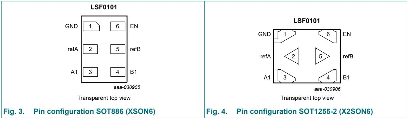
Fig. 3. Pin configuration SOT886 (XSON6)
