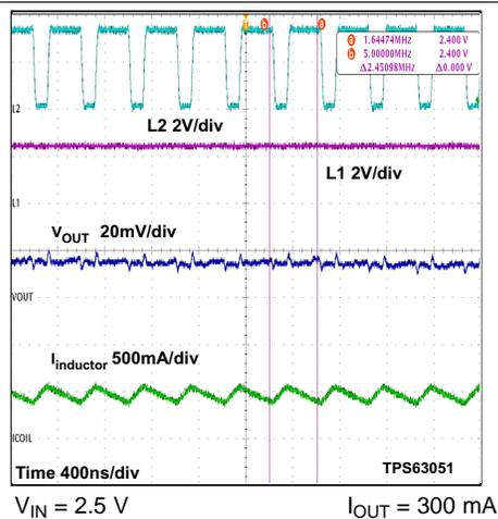
Figure 26. Switching Waveform in Boost Mode and PWM
