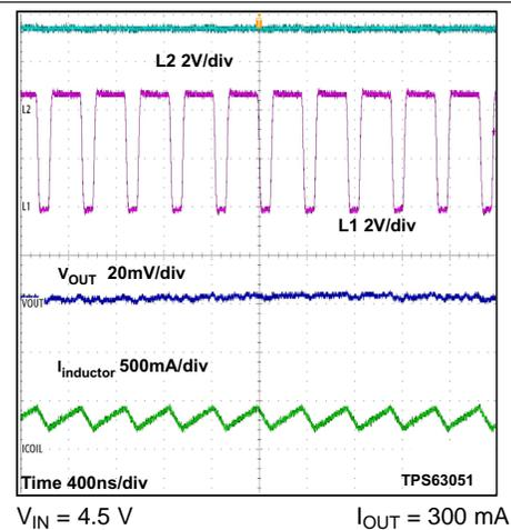
Figure 27. Switching Waveform in Buck Mode and PWM
