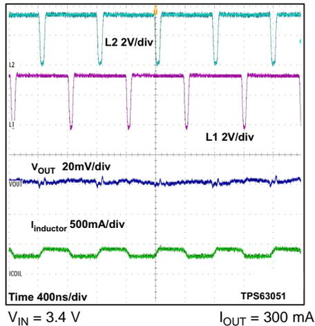
Figure 28. Switching Waveform in Buck-Boost Mode and PWM
