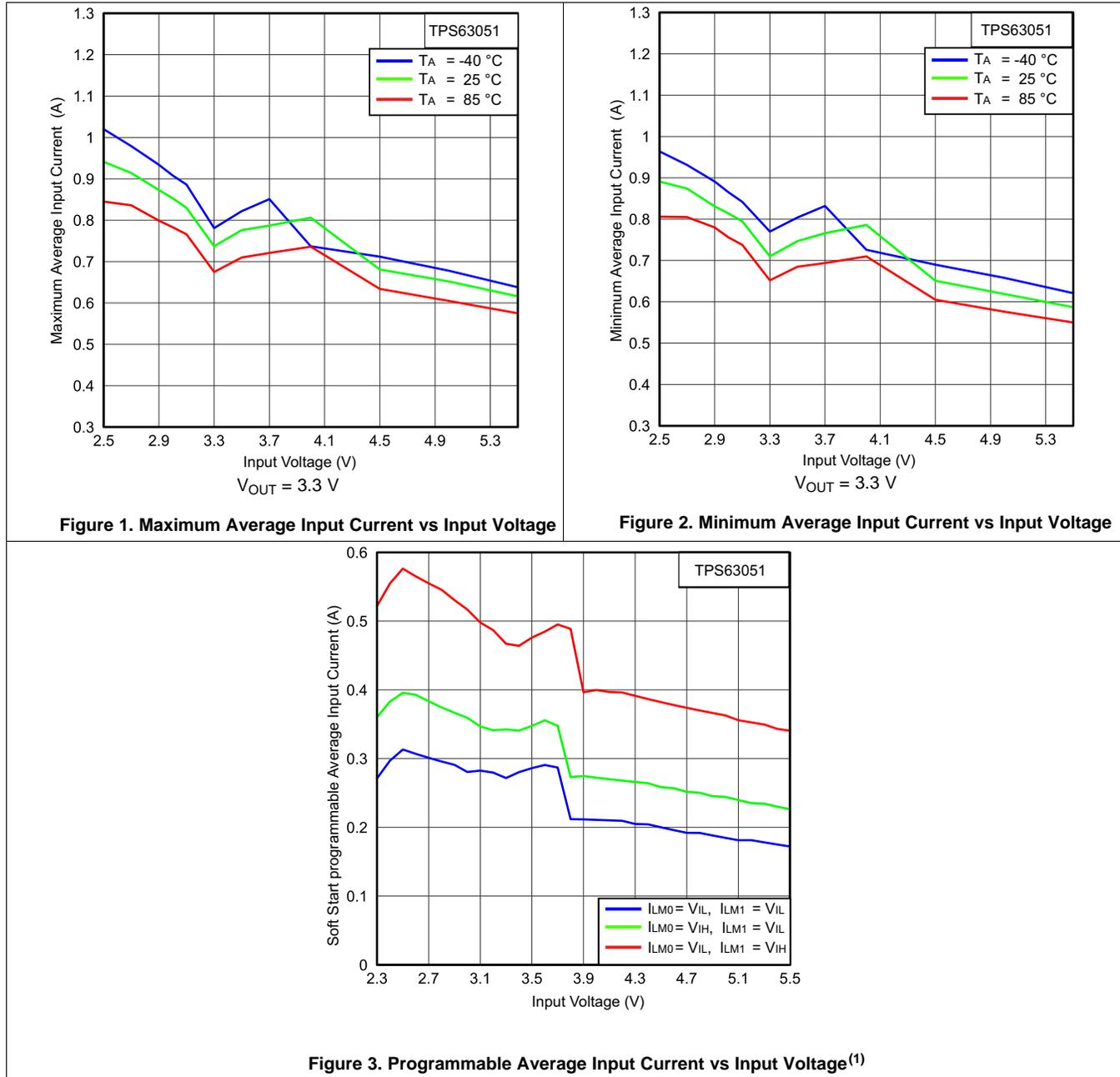
(1) All options only available with the DSBGA package. For VQFN package  $I_{LM1}$  is internally connected to voltage level  $> V_{IH}$
