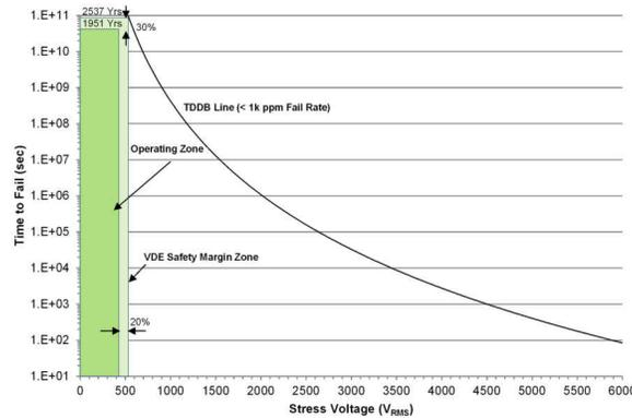
**Figure 9-1. Insulation Lifetime**
