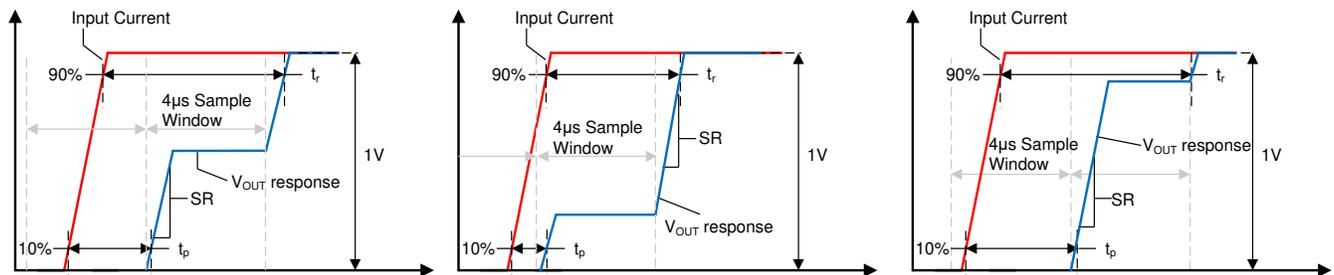
**Figure 8-3. Small Current Input Step Transient Response**
