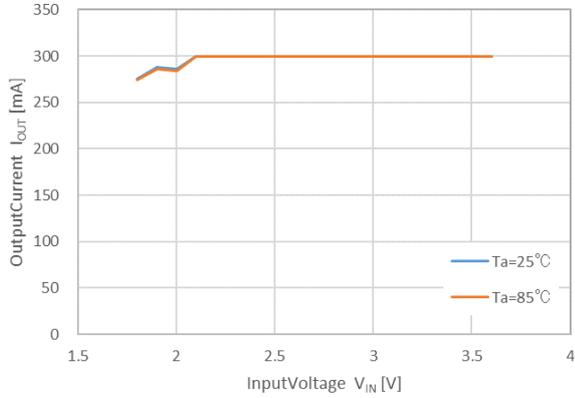
RP605x33xx,  $V_{IN} = 1.8$  to  $5.5V$ ,  $I_{OUT} = (I_{IN} = 300mA)$
