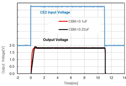
RP605xxx4x,  $V_{IN} = 5.5V$ ,  $T_a = 25^\circ C$
