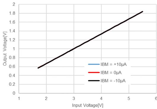
RP605xxx4x,  $V_{IN} = 5.5V$  to Minimum Voltage,  $T_a = 25^\circ C$
