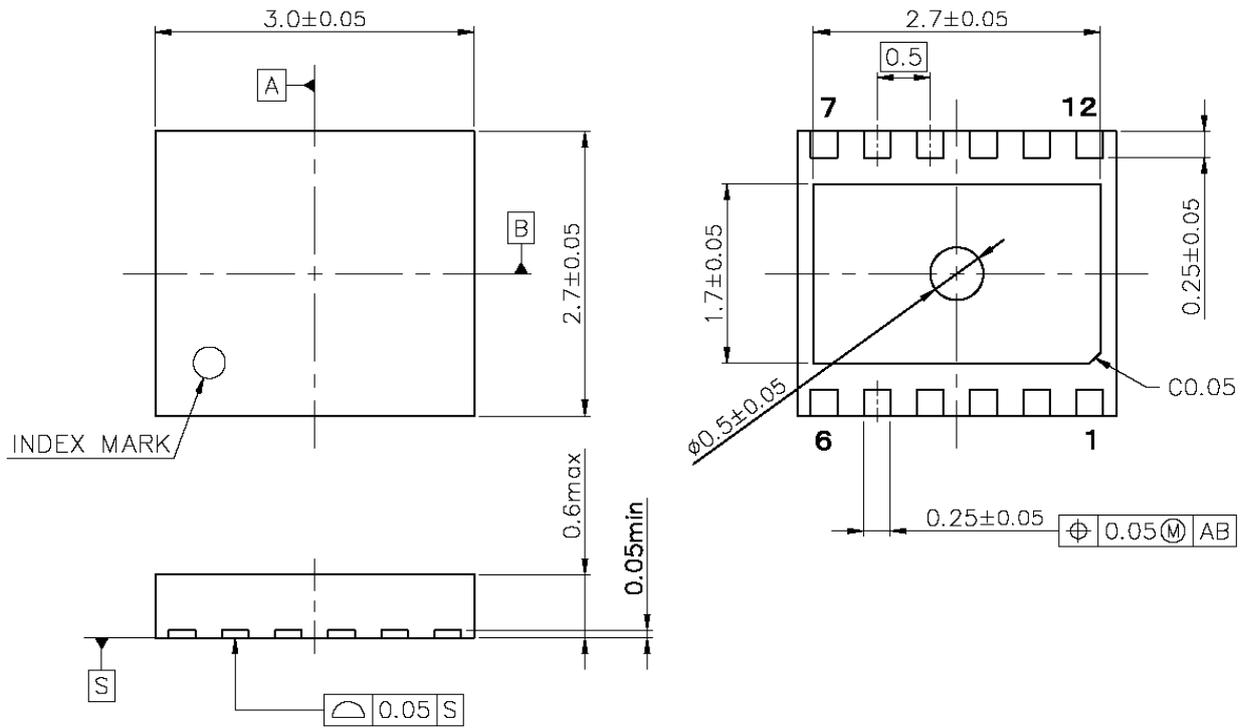
**DFN(PL)2730-12 Package Dimensions (Unit: mm)**
