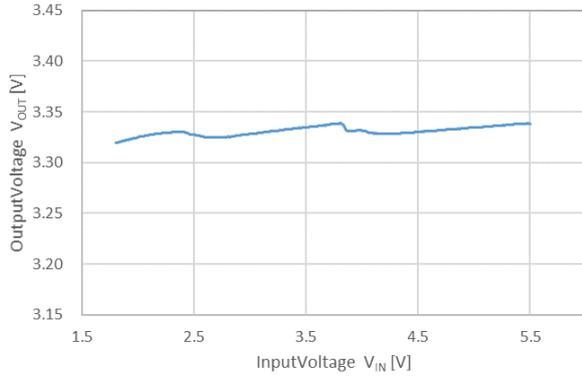
RP605x33xx,  $I_{OUT} = 100\text{mA}$ ,  $T_a = 25^\circ\text{C}$
