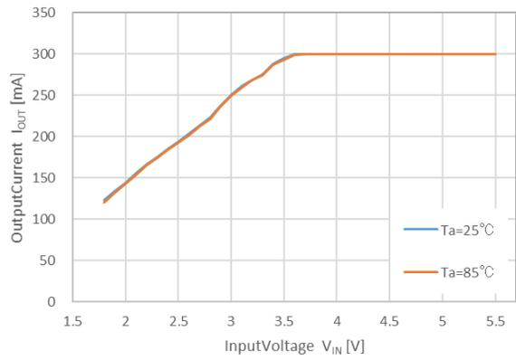
RP605x52xx,  $V_{IN} = 2.3$  to  $5.5V$ ,  $I_{OUT} = (I_{IN} = 300mA)$
