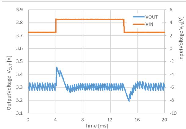
RP605x33xx,  $V_{IN} = 2.5V \leftrightarrow 4.5V$ ,  $I_{OUT} = 100mA$ ,  $T_a = 25^\circ C$
