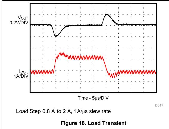
Figure 18. Load Transient
