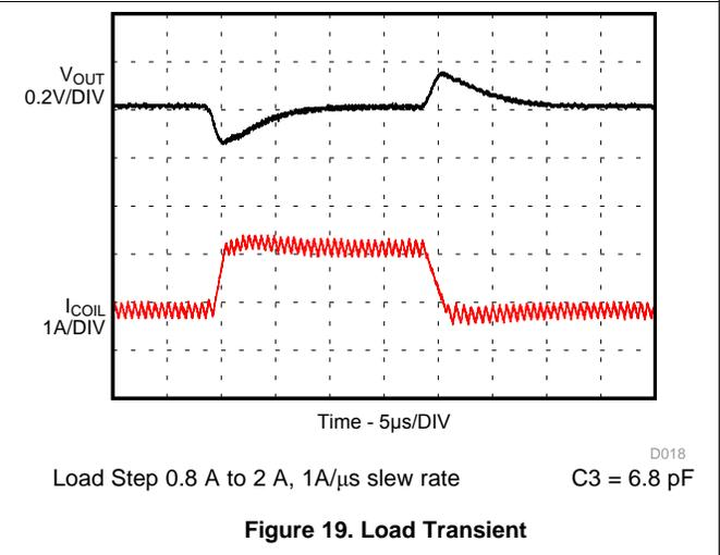
Figure 19. Load Transient
