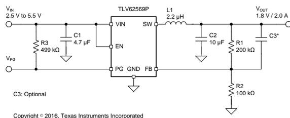
At medium to heavy loads, the device operates in pulse width modulation (PWM) mode with 1.5-MHz switching frequency. At light load, the device automatically enters Power Save Mode (PSM) to maintain high efficiency over the entire load current range. In shutdown, the current consumption is reduced to less than 2  $\mu$ A.
