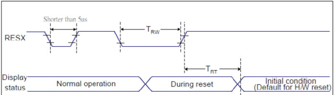
Figure 6.3: Reset Timing
