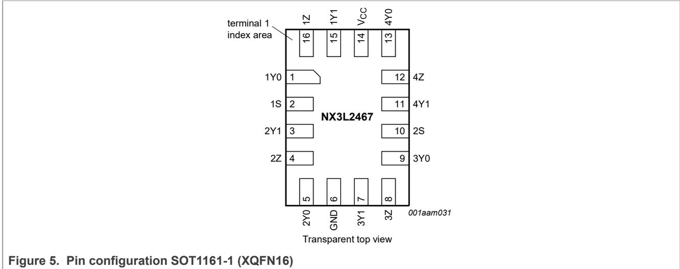
Figure 5. Pin configuration SOT1161-1 (XQFN16)
