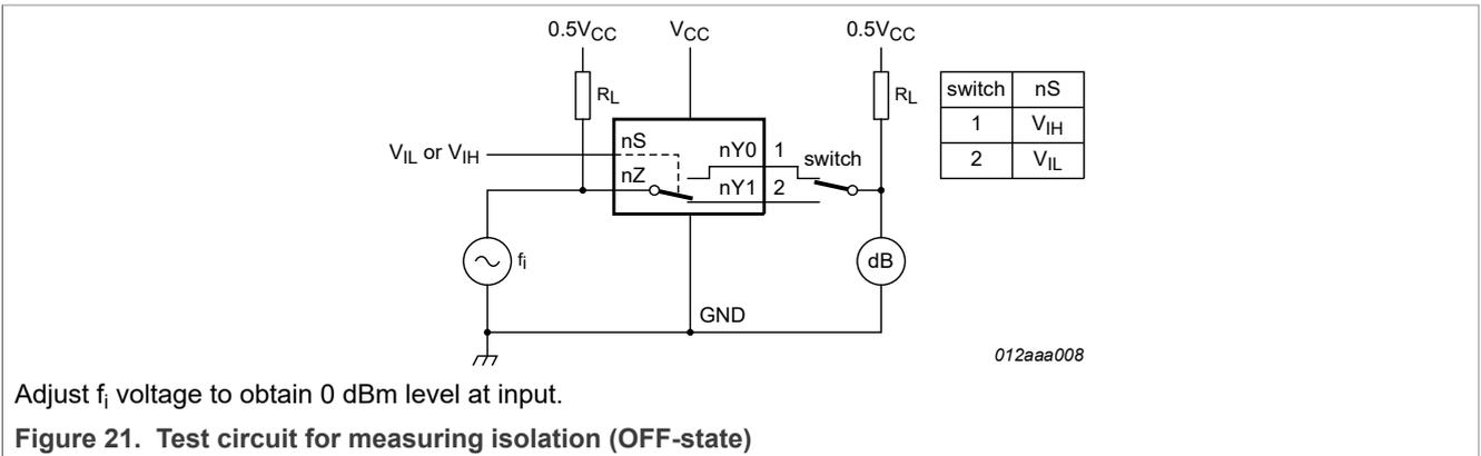
Adjust  $f_i$  voltage to obtain 0 dBm level at input.
