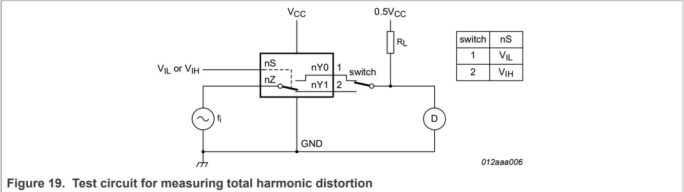
Figure 19. Test circuit for measuring total harmonic distortion
