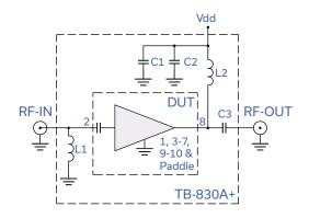
Fig 1. Application and Characterization Circuit
