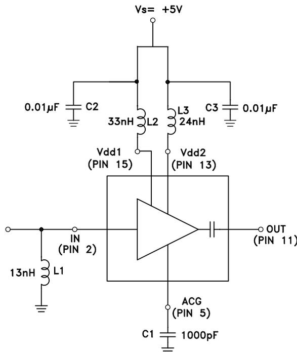
Note: L1, L2, L3 and C1 should be located as close to pins as possible.
