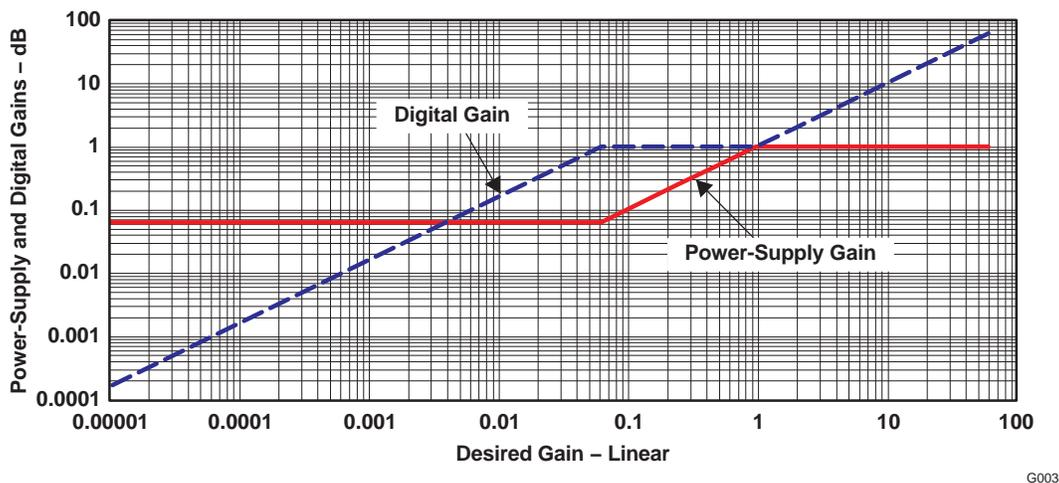
Figure 19. Power-Supply and Digital Gains (Log Space)
