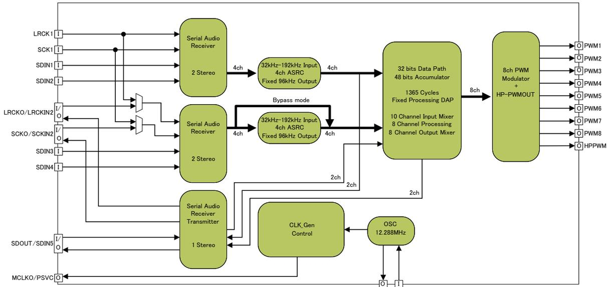
Figure 47. Digital Audio Signal Flow Block Diagram
