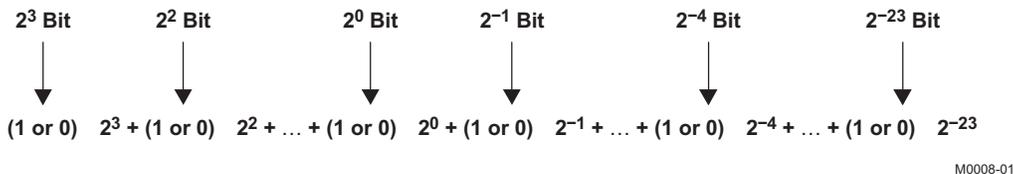
Figure 29. Conversion Weighting Factors—5.23 Format to Floating Point
