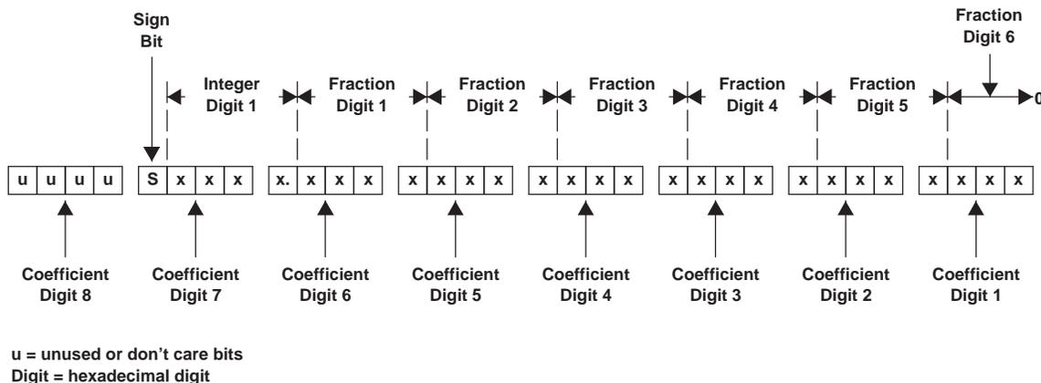
Figure 30. Alignment of 5.23 Coefficient in 32-Bit I<sup>2</sup>C Word
