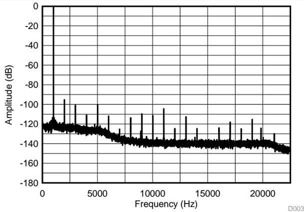
Figure 11. Frequency Response at 44.1 kHz Sampling Rate with -60 dB Input at 1 kHz
