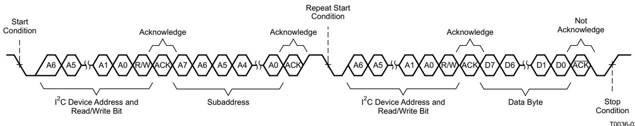
**Figure 43. Single-Byte Read Transfer**
