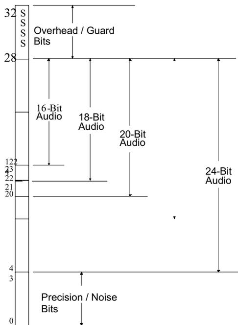
Figure 26. DAP Arithmetic Unit Data Word Structure
