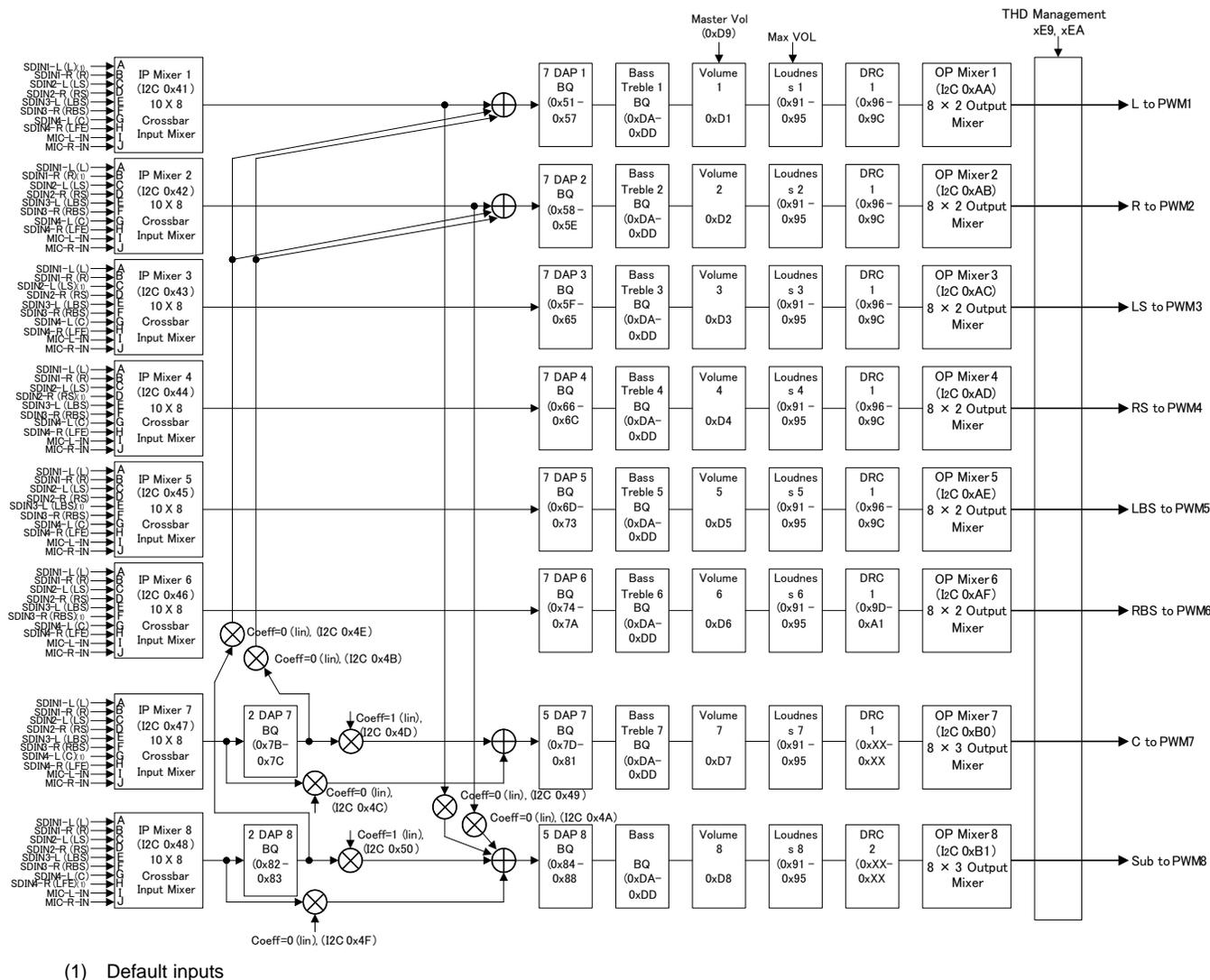
Figure 23. TAS5558 DAP Architecture With I<sup>2</sup>C Registers ( $f_s \leq 96$  kHz)
