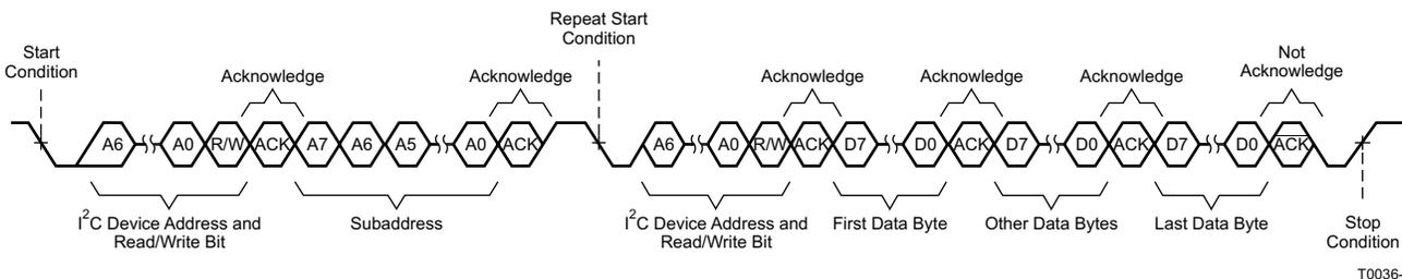
**Figure 44. Multiple-Byte Read Transfer**
