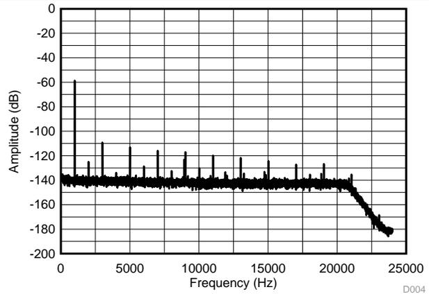
Figure 12. Frequency Response at 44.1 kHz Sampling Rate with 3 dB Input at 1 kHz
