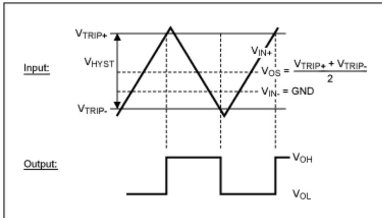
Figure 1. Switch thresholds, hysteresis, and offset voltage.
