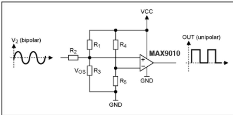
Figure 5. Unipolar comparator with bipolar input signal.
