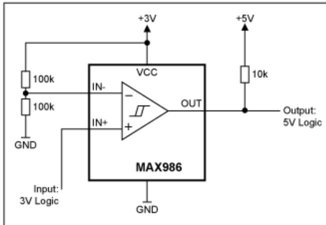
Figure 4. Level translation from 3V to 5V logic.
