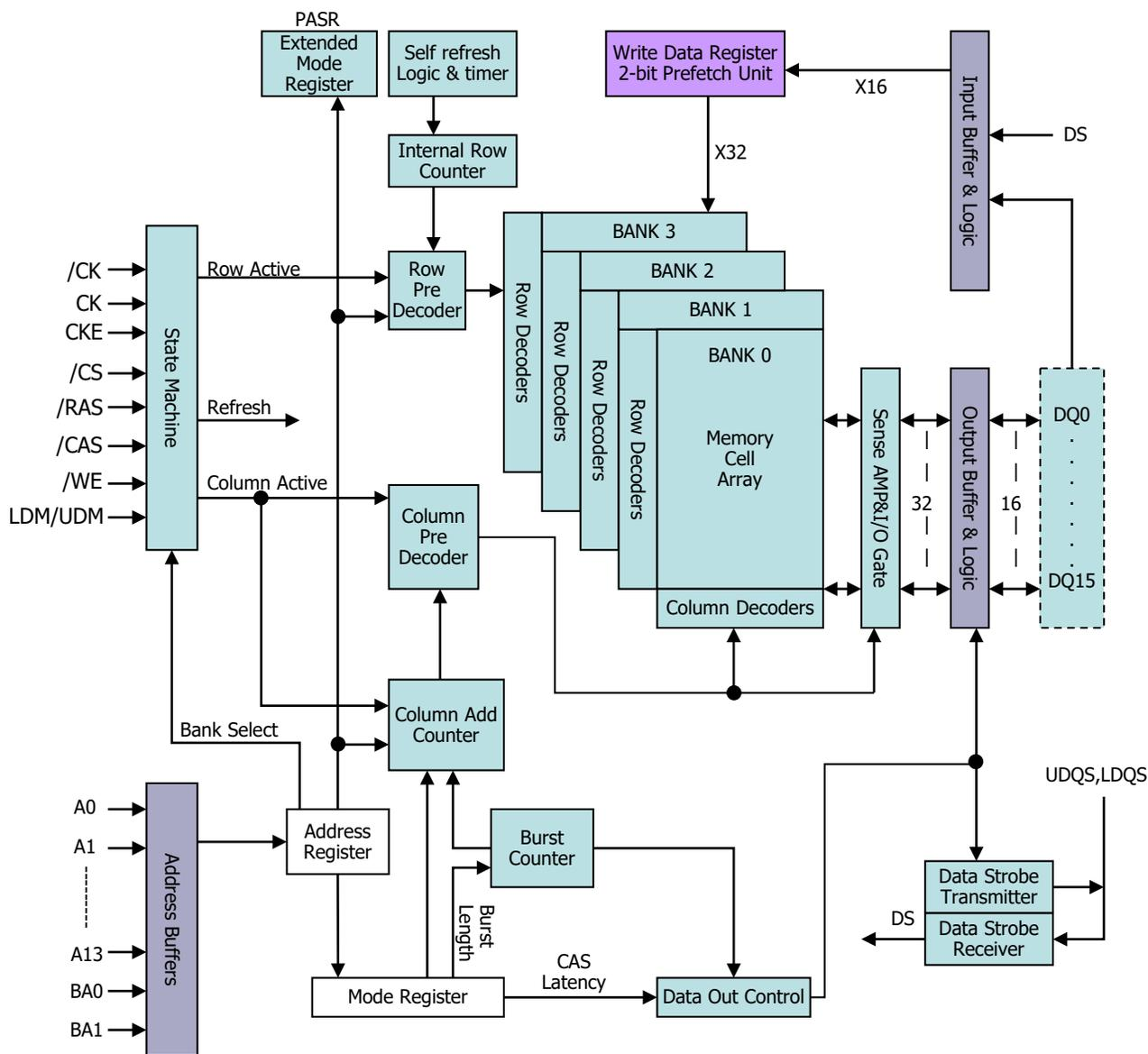
Figure 2.2 : Functional Block Diagram (32Mb X 32)
