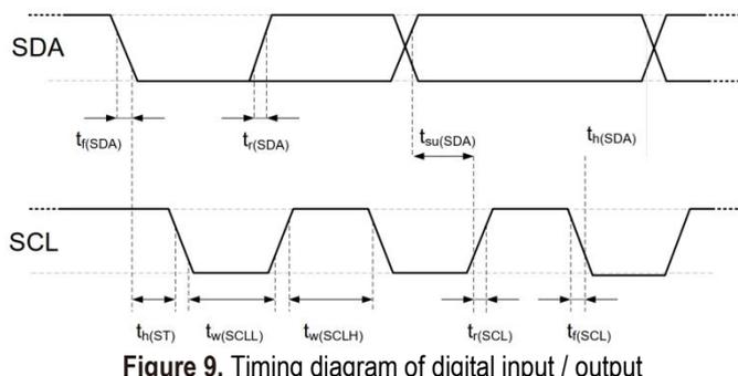
Figure 9. Timing diagram of digital input / output
