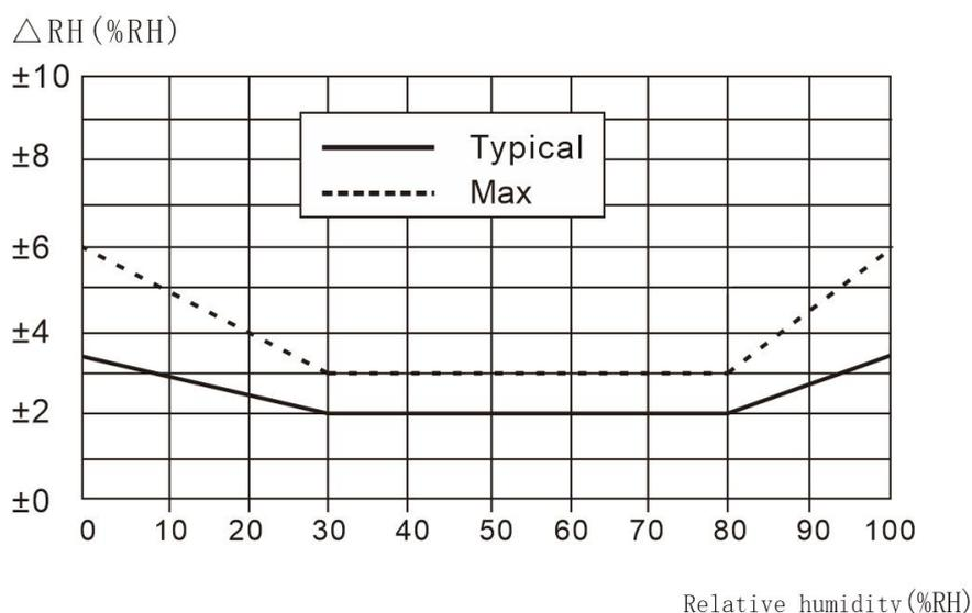
Figure 2. Typical and maximum humidity errors
