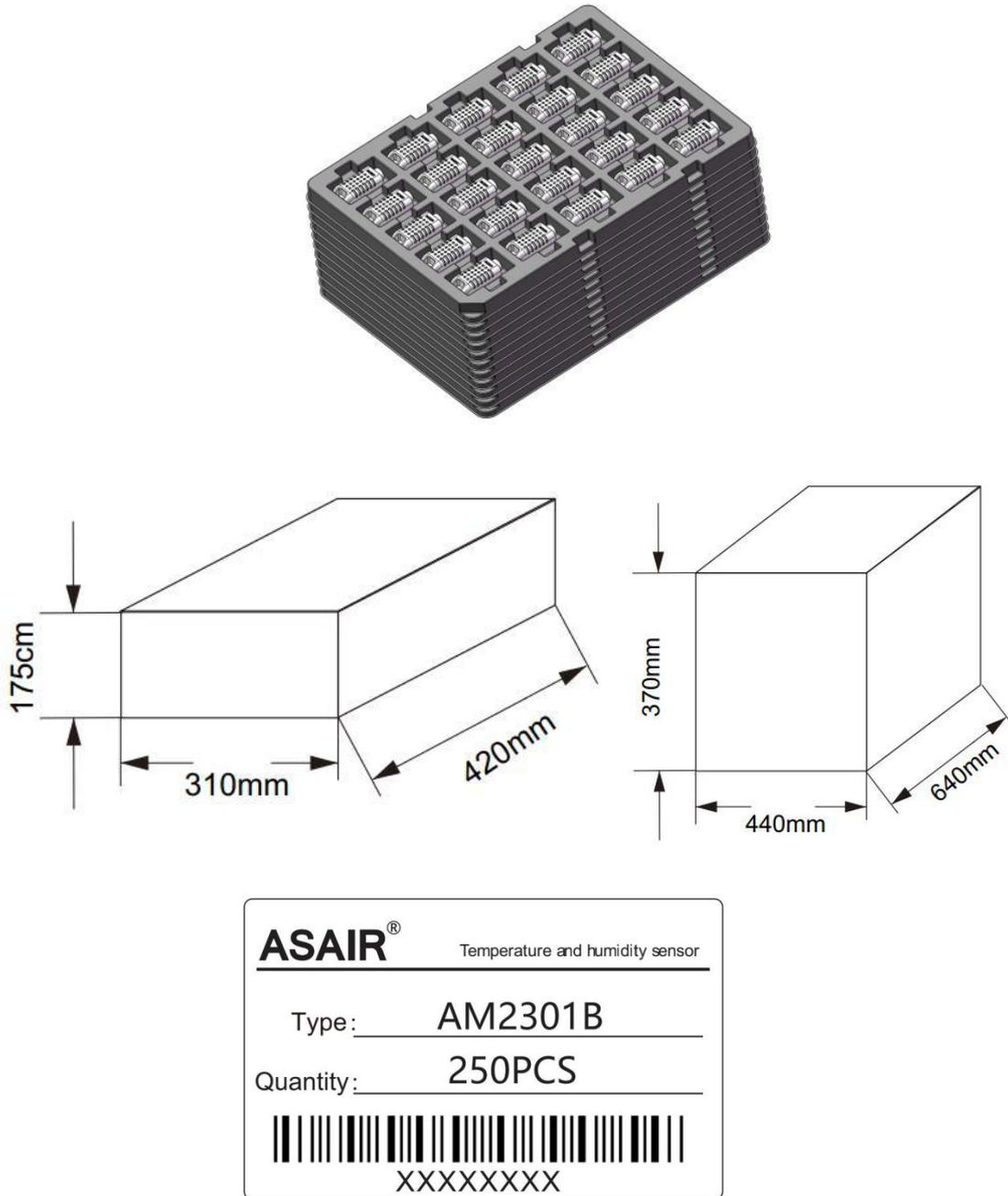
Figure 14. Schematic diagram of packaging
