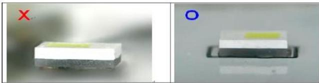
The void rate of the solder on heat transparent lower than 10% is recommended.
