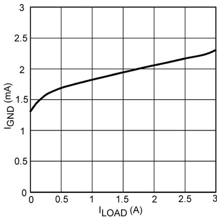
Figure 3.  $I_{GND}$  vs Load Current
