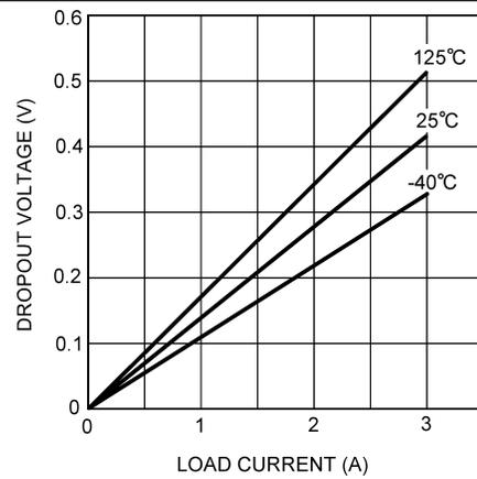
Figure 6. Dropout Voltage vs Load Current
