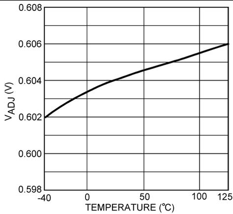
Figure 5.  $V_{ADJ}$  vs Temperature
