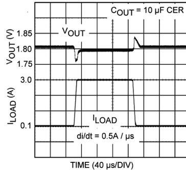
Figure 15. Load Transient Response: 10-μF Ceramic, 0.5-A/μs Di/Dt
