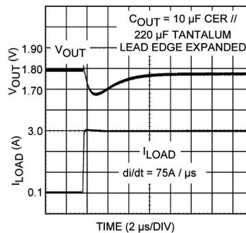
Figure 21. 10- $\mu\text{F}$  Ceramic Paralleled by 220- $\mu\text{F}$  Tantalum
