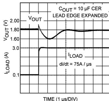
Figure 17. Rising Edge, 10-μF Ceramic, 75 A/μs di/dt
