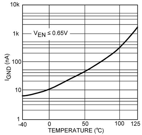
Figure 4.  $I_{GND(OFF)}$  vs Temperature
