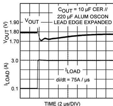
**Figure 22. 10- $\mu\text{F}$  Ceramic Paralleled by 220- $\mu\text{F}$  OSCON**
