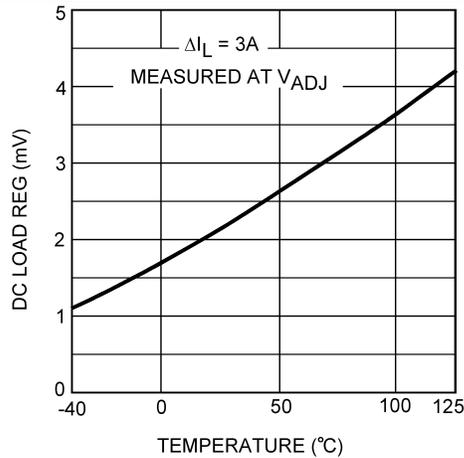
Figure 9. Load Regulation vs Temperature
