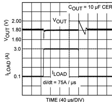
Figure 16. Load Transient Response: 10-μF Ceramic, 75 A/μs di/dt
