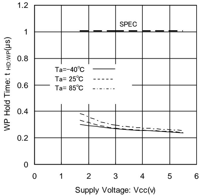
Figure 31. WP Hold Time vs. Supply Voltage
