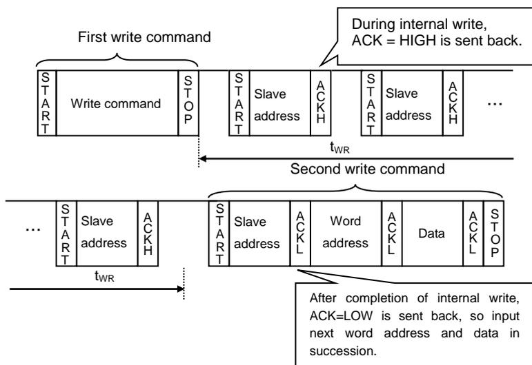
Figure 41. Case of Continuously Write by Acknowledge Polling
