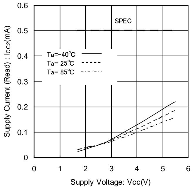
Figure 11. Supply Current (Read) vs. Supply Voltage (f<sub>scl</sub>=400kHz)
