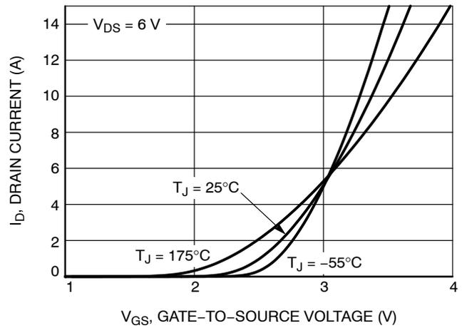
Figure 2. Transfer Characteristics
