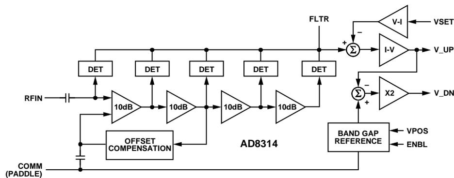
Figure 28. Block Schematic
