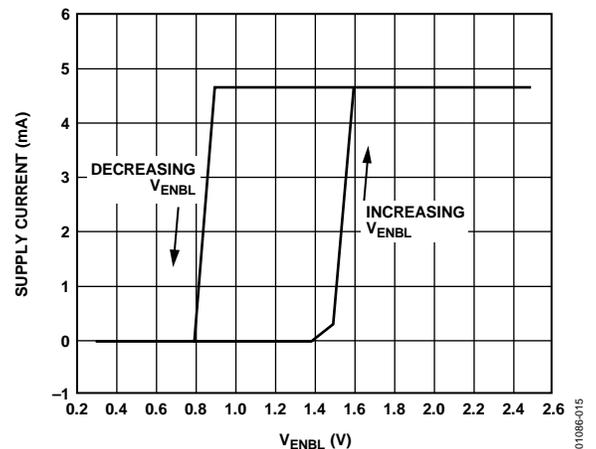
Figure 15. Supply Current vs. ENBL Voltage,  $V_S = 3V$
