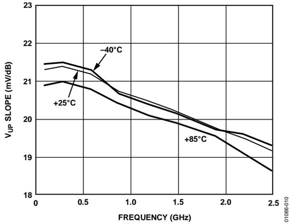
Figure 10. Slope vs. Frequency; -40°C, +25°C, and +85°C
