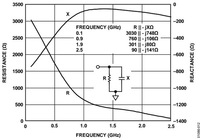
Figure 12. Input Impedance
