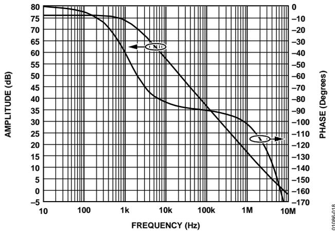
Figure 18. AC Response from VSET to  $V_{DN}$
