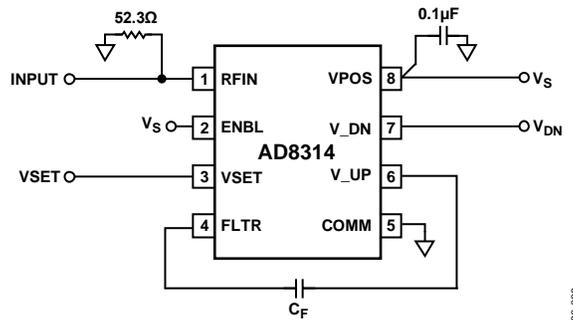
Figure 33. Basic Connections for Operation in Controller Mode
