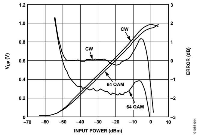
Figure 44. Shift in Transfer Function due to 64 QAM
