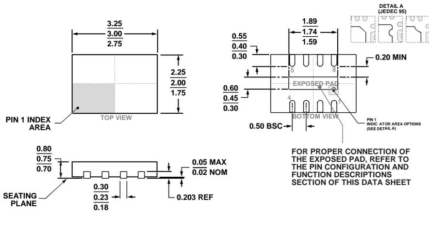
Figure 49. 8-Lead Lead Frame Chip Scale Package [LFCSP] 2 mm x 3 mm Body and 0.75 mm Package Height (CP-8-23)
