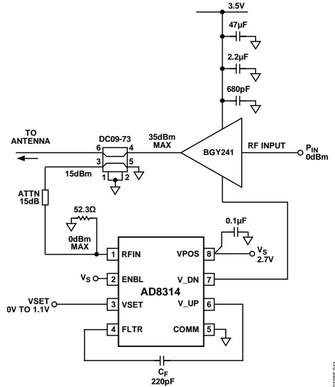
Figure 41. A Single Mode Power Amplifier Control Circuit
