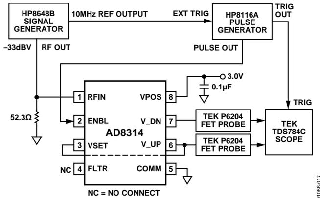
Figure 17. Test Setup for ENBL Response Time
