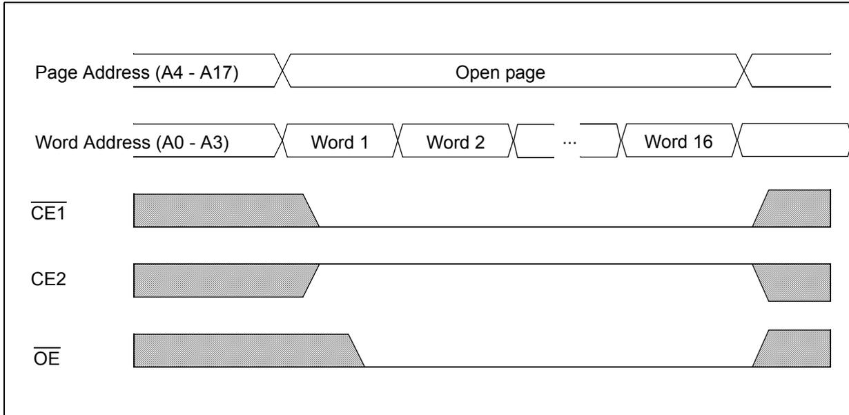
Note: Page mode operation is a method of addressing the SRAM to save operating current. The internal organization of the SRAM is optimized to allow this unique operating mode to be used as a valuable power saving feature.
