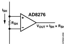
Figure 51. AD8276 Monitoring Current Through a Shunt Resistor
