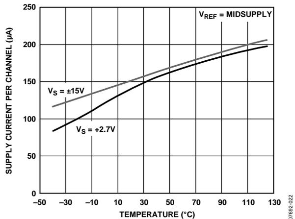
Figure 25. Supply Current Per Channel vs. Temperature
