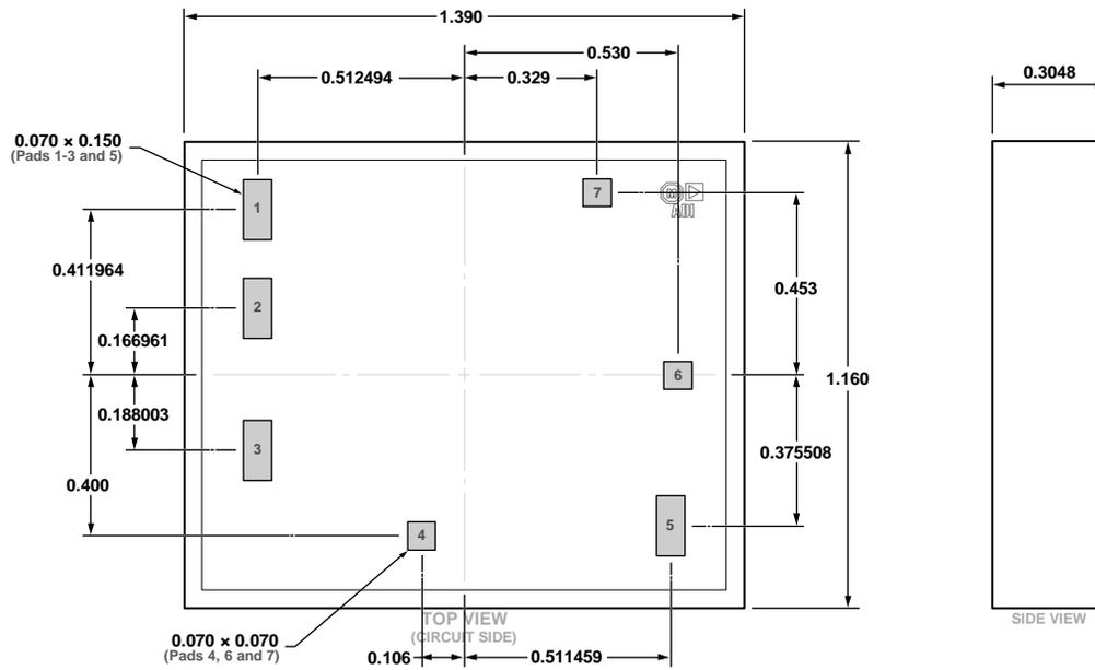
Figure 56. 7-Pad Bare Die [CHIP]
