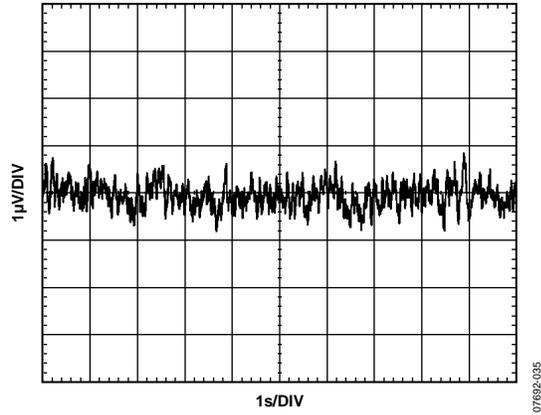
Figure 37. 0.1 Hz to 10 Hz Voltage Noise
