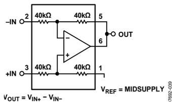
Figure 43. Difference Amplifier, Gain = 1, Referenced to Midsupply
