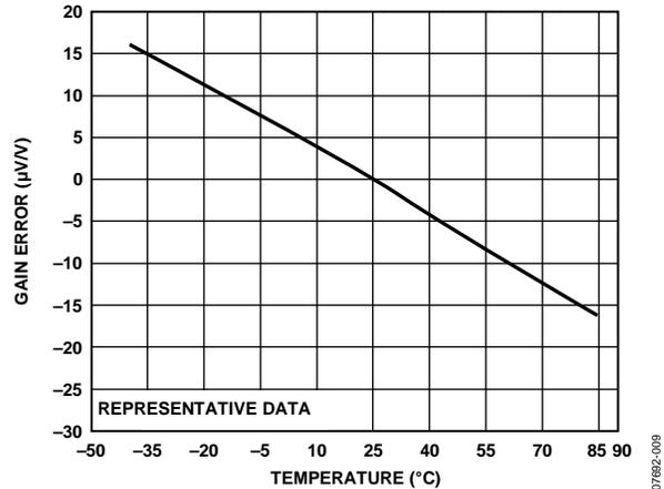
Figure 12. Gain Error vs. Temperature, Normalized at 25°C
