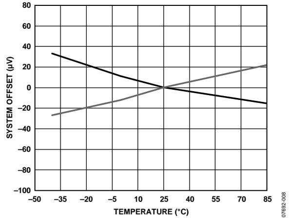
Figure 11. System Offset vs. Temperature, Normalized at 25°C
