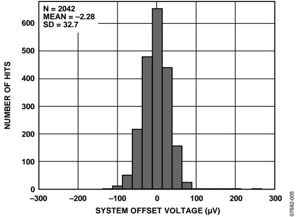
Figure 8. Distribution of Typical System Offset Voltage
