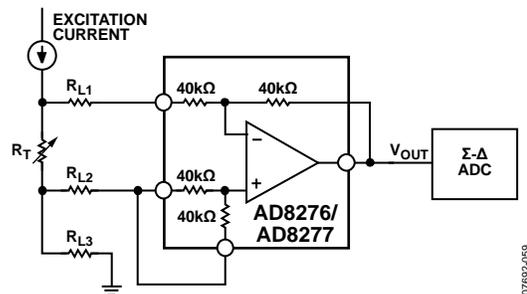
Figure 53. 3-Wire RTD Cable Resistance Error Measurement
