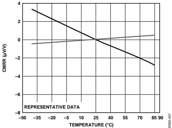
Figure 10. CMRR vs. Temperature, Normalized at 25°C
