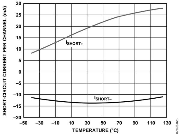
Figure 26. Short-Circuit Current Per Channel vs. Temperature
