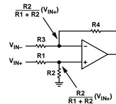
Figure 39. Voltage Division in the Difference Amplifier Configuration
