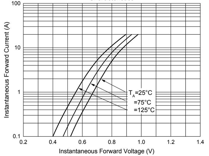
Fig. 5 - MBR10200CTH Typical Instantaneous Forward Characteristics
