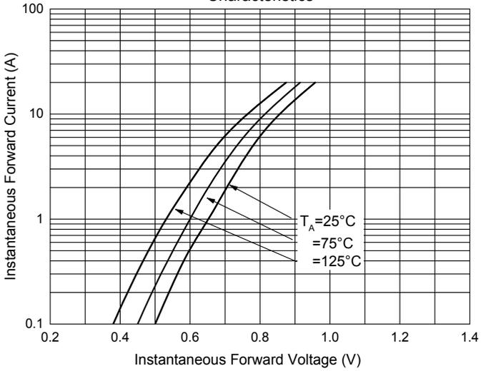
Fig. 4 - MBR10150CTH Typical Instantaneous Forward Characteristics
