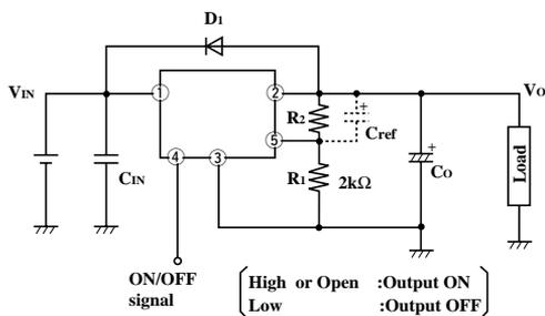
D1 : This device is necessary to protect the element from damage when reverse voltage may be applied to the regulator in case of input short-circuiting.
