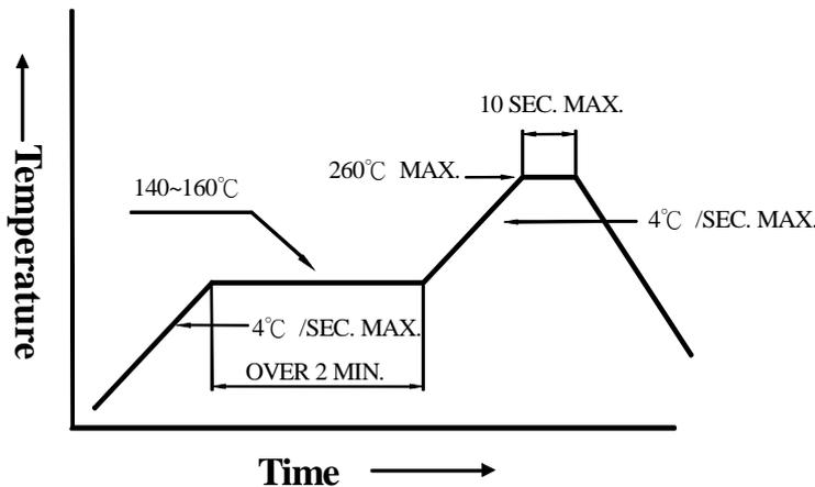
3. DIP soldering (Wave Soldering) :
