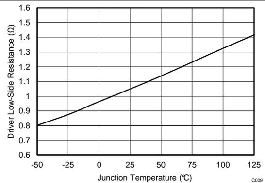
Figure 10. Driver Pull Down Resistance vs Junction Temperature
