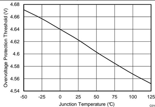
Figure 11. Over Voltage Protection Threshold vs Junction Temperature
