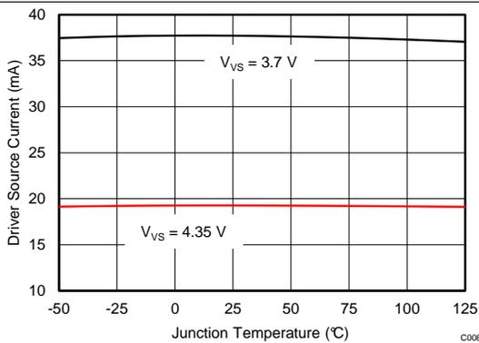
Figure 9. Driver Output Source Current vs Junction Temperature
