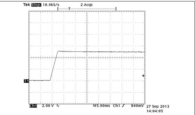
Figure 21. Output at Startup 115-V RMS, No Load
