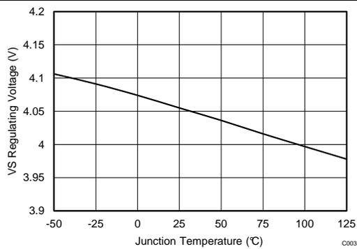
Figure 3. VS Pin Regulation Voltage vs Junction Temperature
