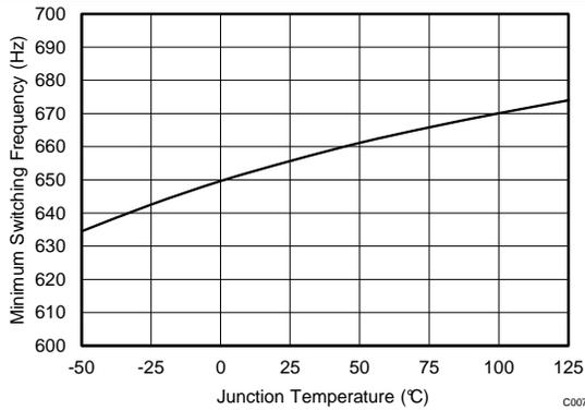
Figure 7. Minimum Switching Frequency vs Junction Temperature
