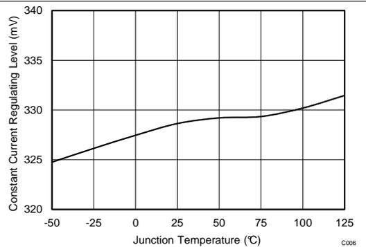
Figure 6. Constant Current Regulation Level vs Junction Temperature
