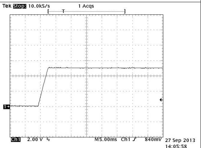
Figure 23. Output at Startup 230-V RMS, No Load
