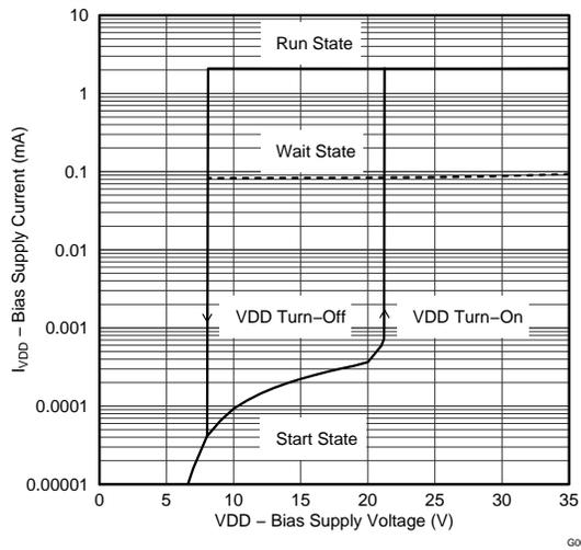
Figure 1. Bias Supply Current vs VDD Voltage
