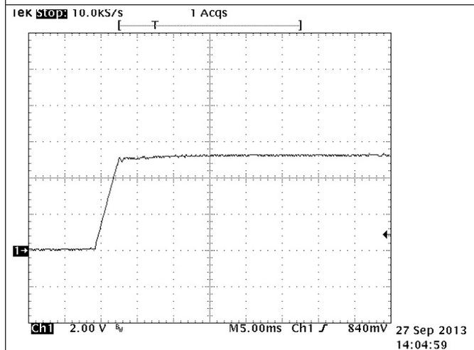
Figure 22. Output at Startup 115-V RMS, 5-Ω Load
