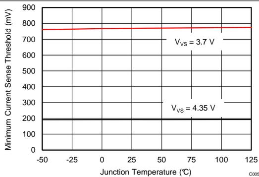
Figure 5. Current Sense Threshold vs Temperature
